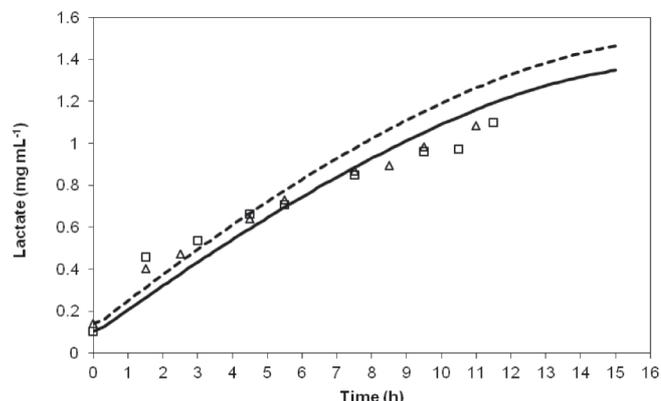
Fig. 3 – Evolution of product concentrations (samples taken from the bottle). Experimental data with (□) and without (Δ) antibiotics and, the results of modelling with (continuous line) and without (discontinuous line) antibiotics (eq. 11 to 14, and 19 to 22).
