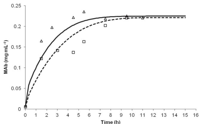
Fig. 4 – Evolution of antibody concentration (samples taken from the bundle). Experimental data with ( $\square$ ) and without ( $\Delta$ ) antibiotics and, the results of modelling with (continuous line) and without (discontinuous line) antibiotics (eq. 11 to 14, and 19 to 23).
