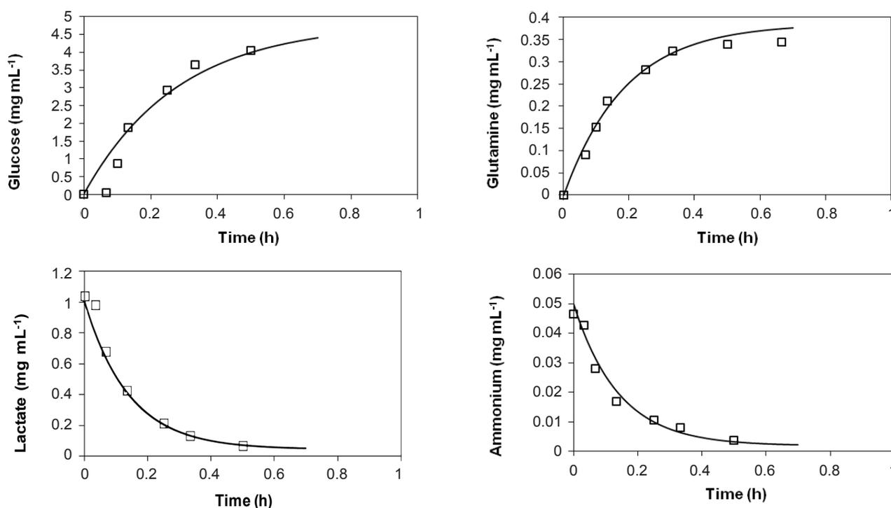
Fig. 5 – Evolution of substrate and product concentrations in diffusion assays (samples taken from the bundle). Experimental data ( $\square$ ) and the results of modelling (continuous line) (eq. 11 to 18; reaction term being null).
