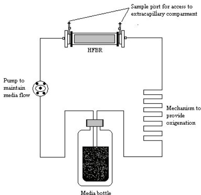
Fig. 1 – Schematic representation of the HFBR system
