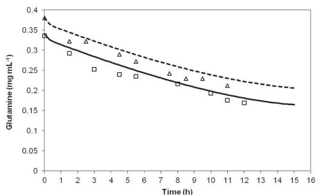
Fig. 2 – Evolution of substrate concentrations (samples taken from the bottle). Experimental data with (□) and without (Δ) antibiotics, and the results of modelling with (continuous line) and without (discontinuous line) antibiotics (eq. 11 to 14, and 19 to 22).
