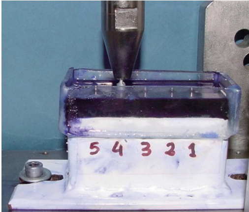
Fig. 1. Working model and compressive cyclic load test.
