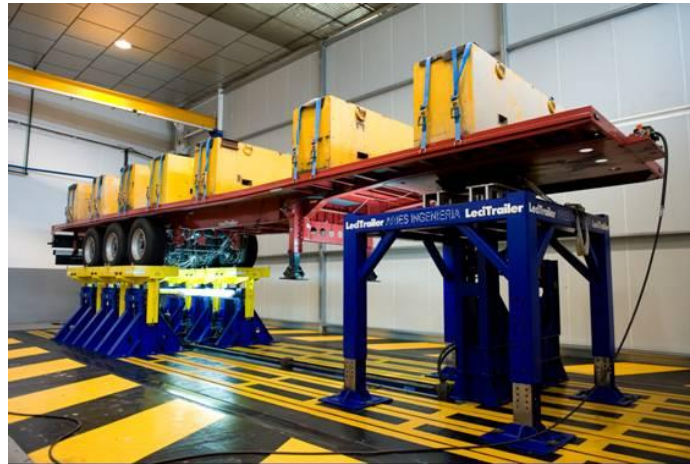
Figure 1. Fatigue test bench for semi-trailers developed for this study
