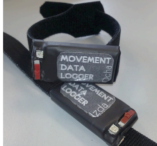
(b) The bracelets capacity allows the store of data from up to 45 minutes and the data can be consequently downloaded to a computer.
