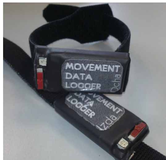
Figure 4 The tri-axial bracelets used in this study, one for each hand.
