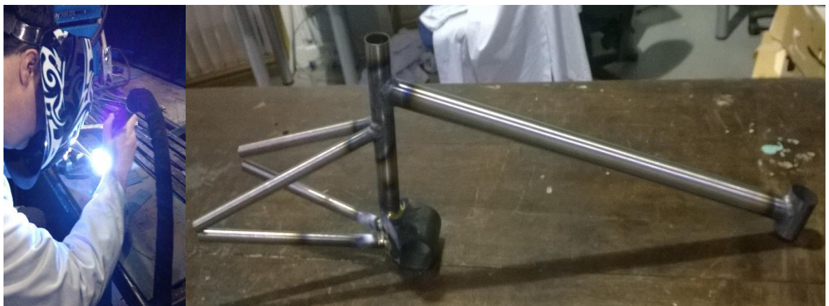
Figure 26 - Welding of Main Frame
