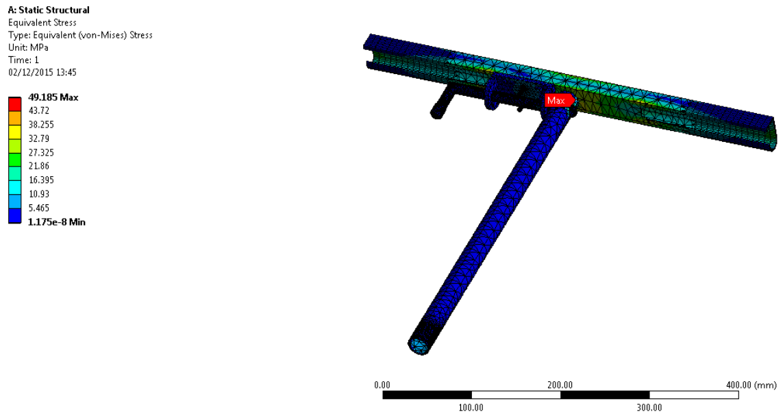
Figure 21 - ANSYS Stress Analysis of Handlebars
