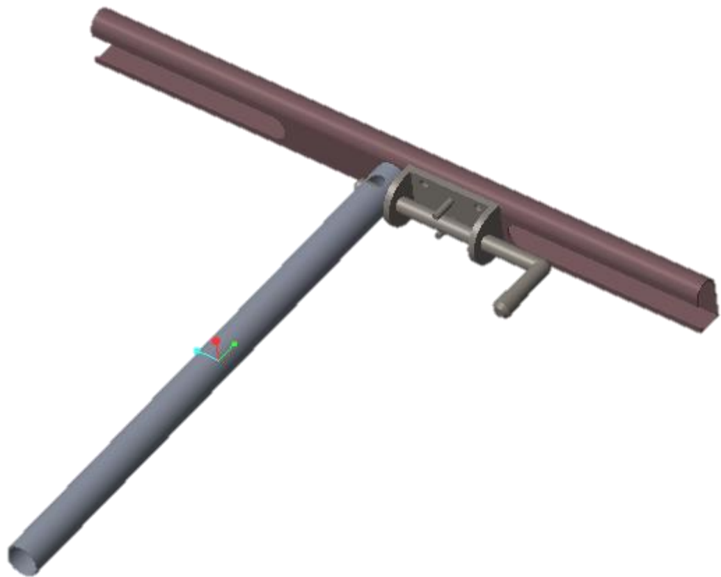
Figure 18 - Assembly of Upper Steering Column and Handlebars
