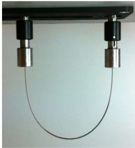
Fig. 30. Chuck-to-chuck method set-up [22]
