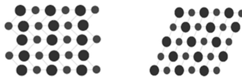
Fig. 3. Twinned martensite on the left and detwinned martensite on the right [1]
