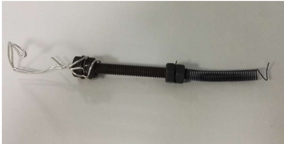
Fig. 48. Measurement of the initial length ( L_0 ) of spring 1. Close-up to the clamping system on the side of the hook; the end of the wire passes through the groove machined on the nut and compressed but another nut.
