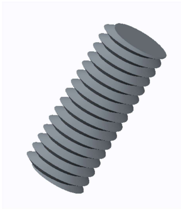
Fig. 64. Clamping system: Creo Parametric model of the teflon bolt
