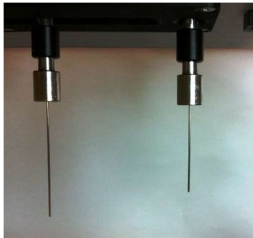
Fig. 32. Uneven failure of the wire in the chuck-to-chuck method [22]
