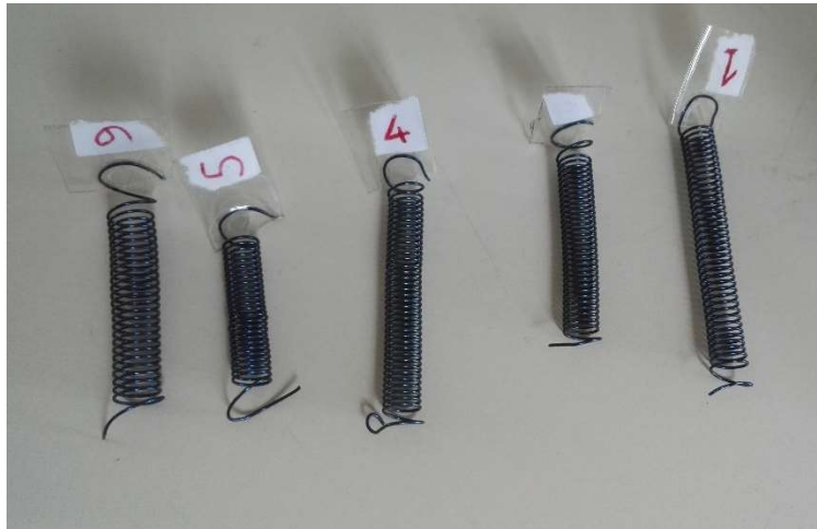
Fig. 46. Obtained springs after the heat treatment
