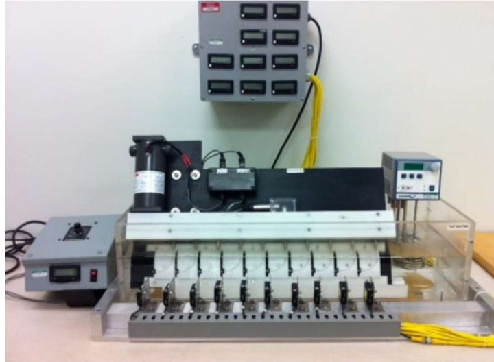
Fig. 35. Machined block method complete set-up [22]
