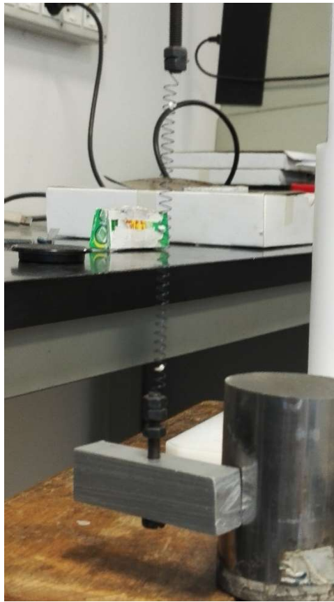
Fig. 51. Spring 3 loaded. The two marks made with teflon can be observed (two white points)
