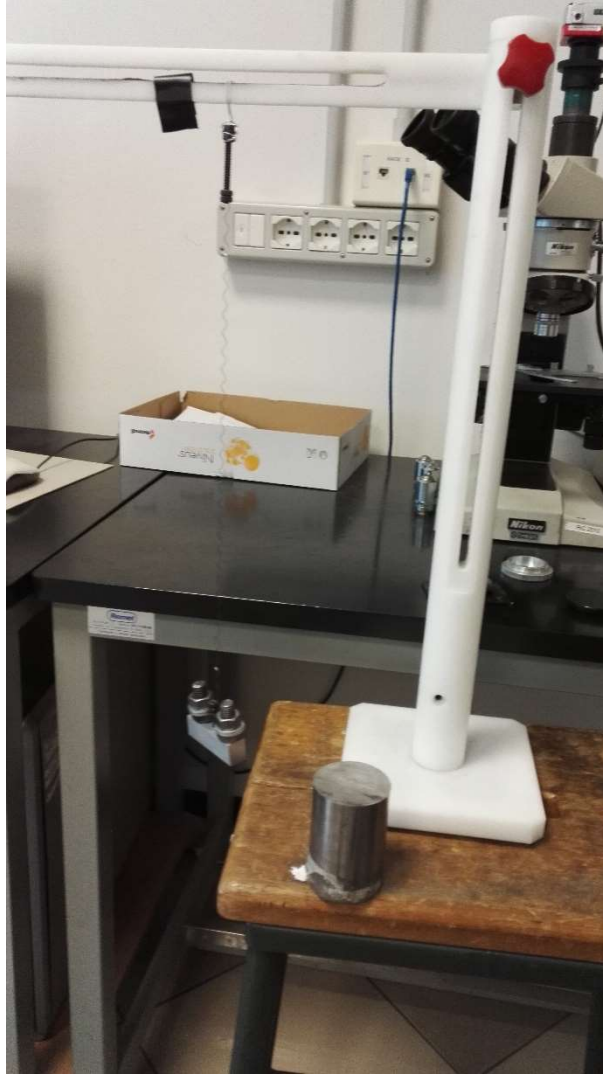
Fig. 52. Spring 3 loaded with the maximum weight. Significant deformation observed.
