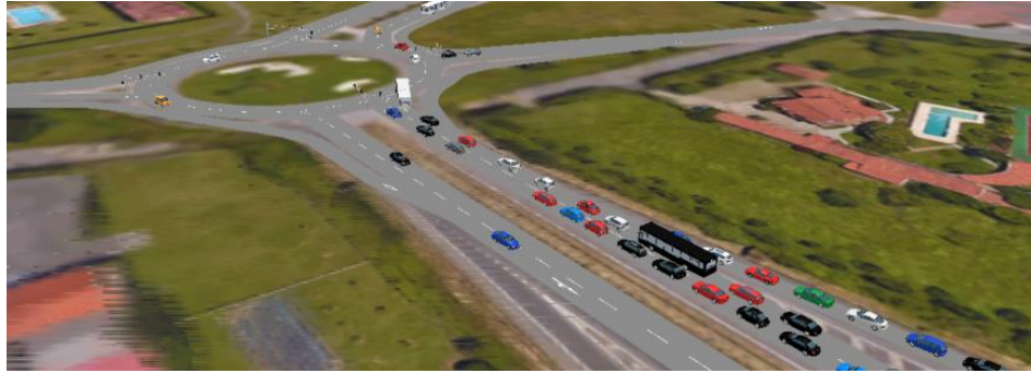
Figure 9.4. Queue formed in Highway entrance
