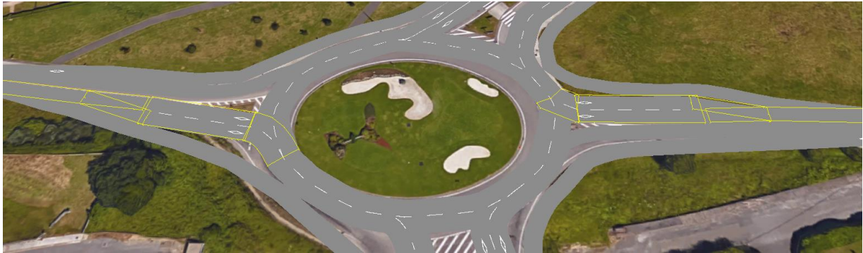
Figure 8.2. Flaring of Viesques and Polytechnic entrances
