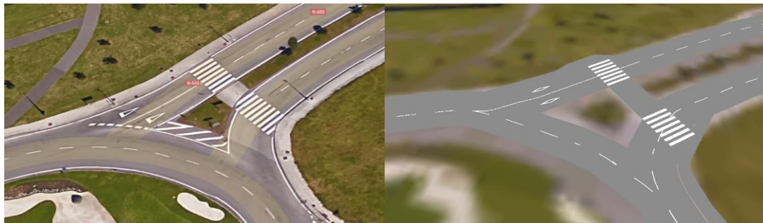
Figure 4.37. Zebra crossing in Molinón Stadium entrance in the reality (left) and in the model (right)
