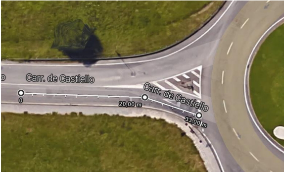
Figure 4.26. Visibility distance measurement in Polytechnic School entrance [Google Earth]
