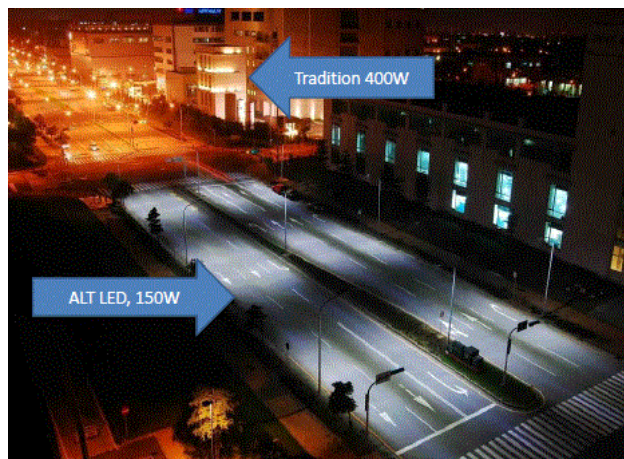
Fig. 1.11. Difference between LED and traditional HPS lamps in street lighting
