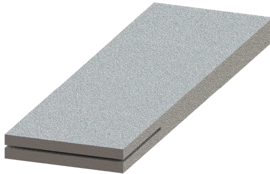
Figura 3.1. Geometría de la probeta SCB “ Split Cantilever Beam ”, SSCB “ Simplified Split Cantilever Beam ” y MSCB “ Modified Split Cantilever Beam ”.
