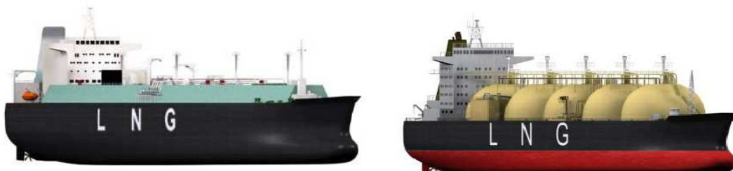
Figure 2-5: Membrane and Moss type LNG carriers
