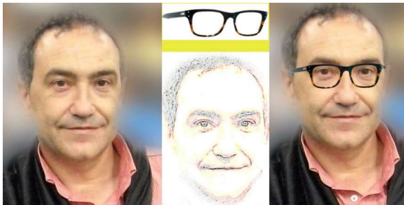
Figure 5 - Photo capture (leftmost) used for the detection of reference points based on face recognition and AR markers (centre) and to superimpose a pair of glasses over the face (rightmost)
