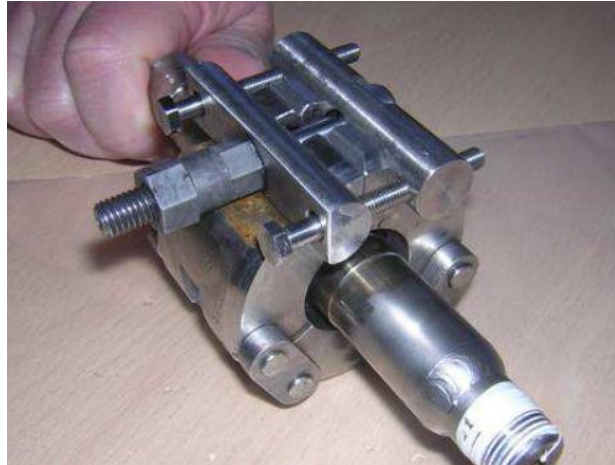
Fig. 18. Reinforcement of the fastener in a QDS [Garlock c].
