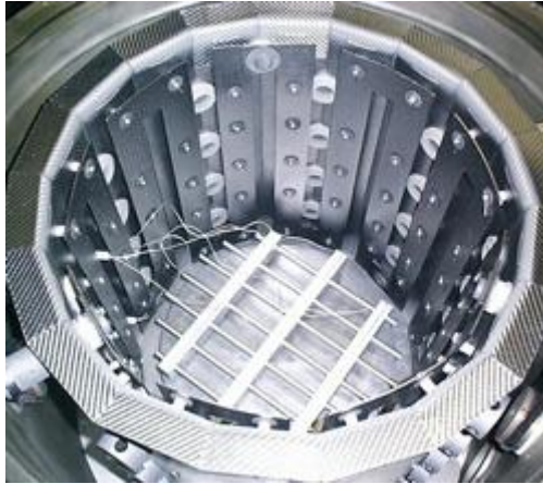
Fig. 26. Interior of a vacuum brazing furnace.
