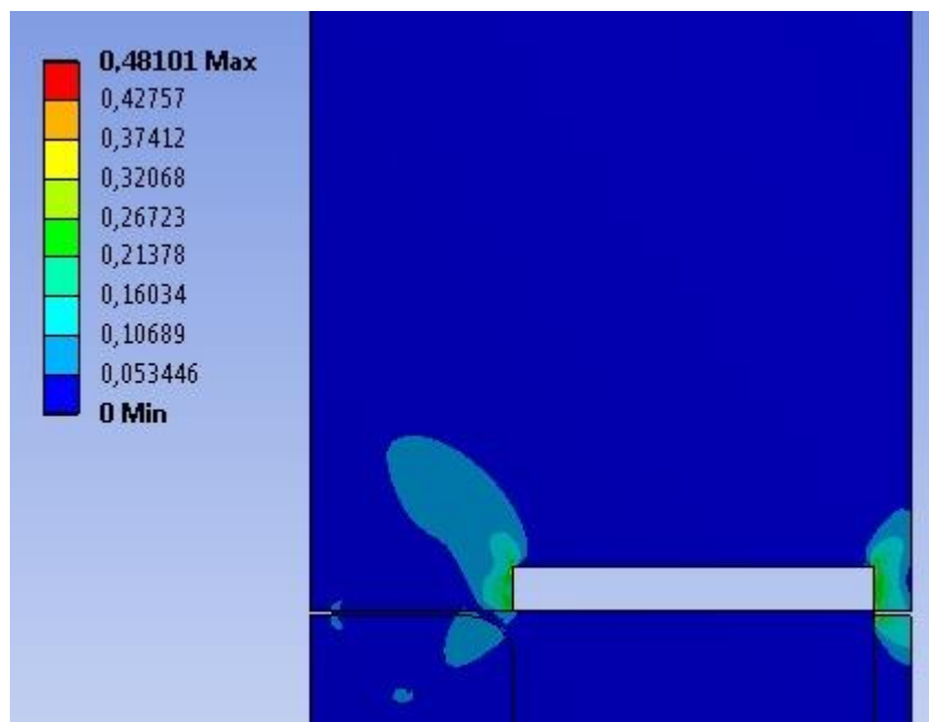
Fig. 36. Equivalent plastic strain at the beginning of the cooling process.
