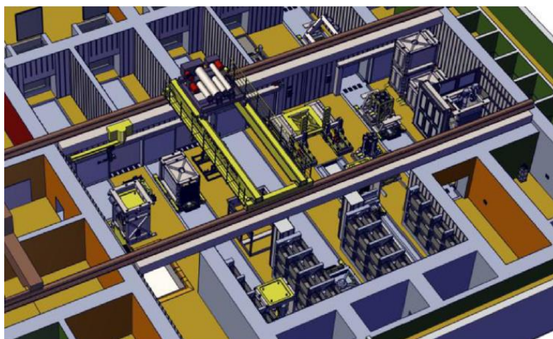
Fig. 16. CEA proposal for HC tooling (ICRH antenna port plug refurbishment) [Fer 13].
