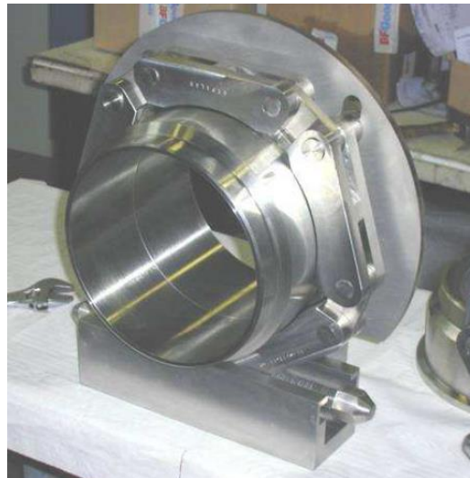
Fig. 17. Support and alignment for QDS [Garlock c].
