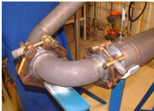
Fig. 15. High temperature QDS (650°C) [Garlock c].
