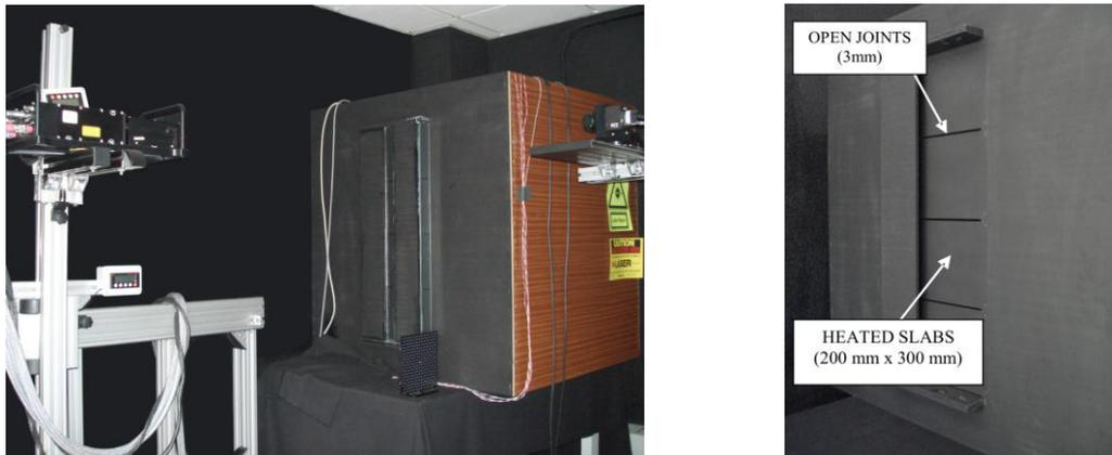
Fig. 1. (a) OJVF experimental model and PIV system; (b) Detail of the slabs of the exterior coat.
