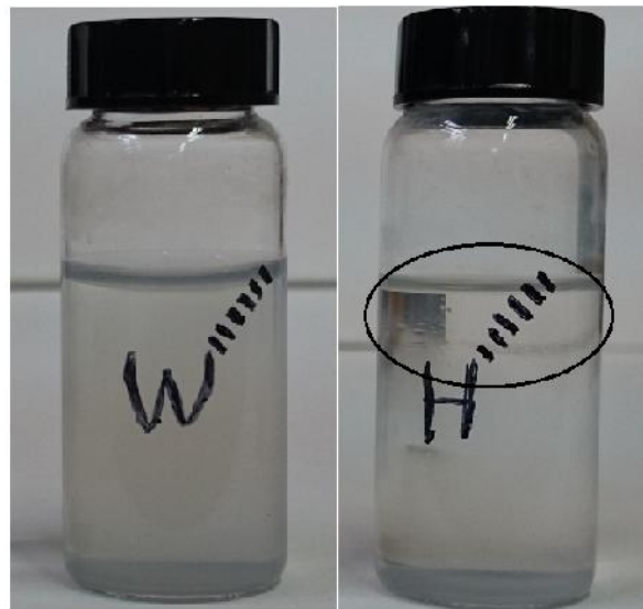
Figure 21: Comparison between ZnO-D (0.025%) dispersion in water (left bottle) and in hexane (right bottle).
