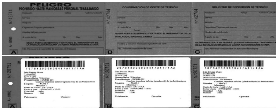
Fig. 1 - Switch off/on cards. traditional format (top) and current format used after SICRET setup (bottom); information is coded in a bar code to be used in the shut down/up process.
