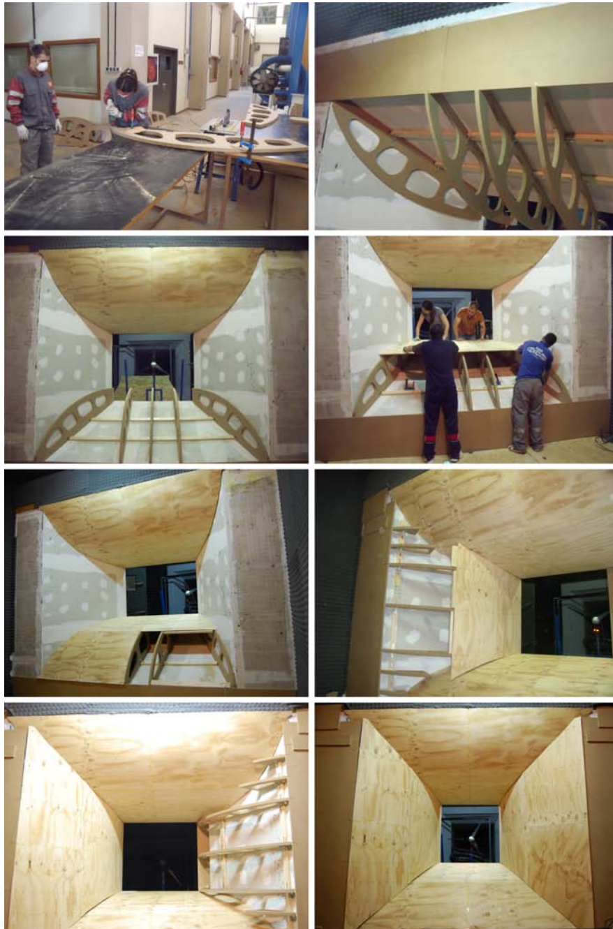
Figure 3.14: Construction process of the nozzle
