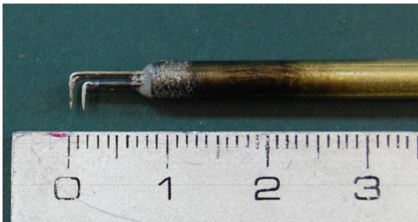
Figure 2.5: Image of a manufactured HW probe for this thesis
