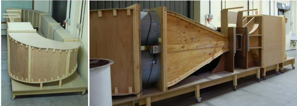
Figure 3.28: Finished closed-loop PIV wind tunnel
