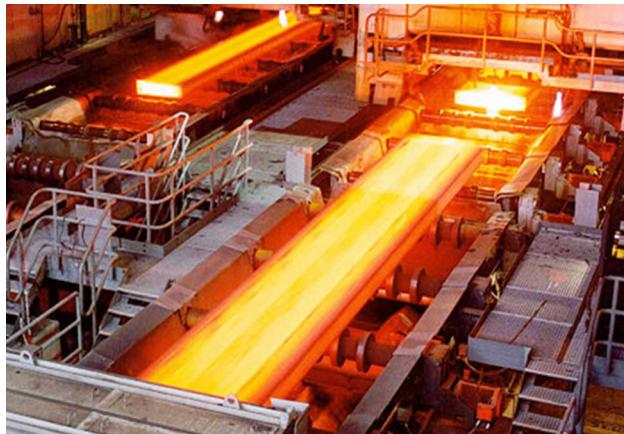
**Fig. 2** Slabs in the continuous casting lines
