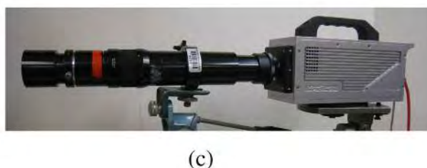
Fig. 1. Schematic of the experimental setup and diagnostic facilities. (a) Drop tube furnace (DTF), (b) three-color optical pyrometer and (c) high speed camera.
