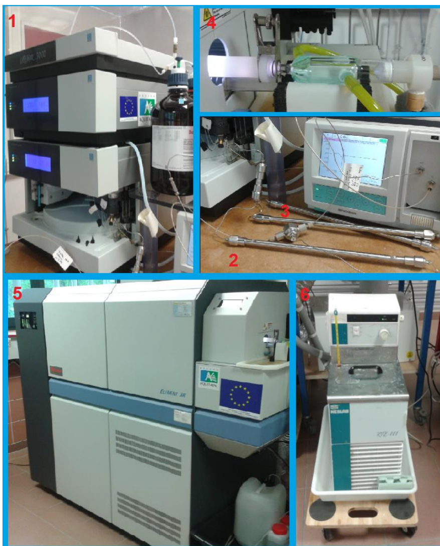
Figure 8. Instrumentation: pump and autosampler (1), GPC columns (2), splitter (3), nebulizer (4), ICP-MS (5) and temperature controller (6).
