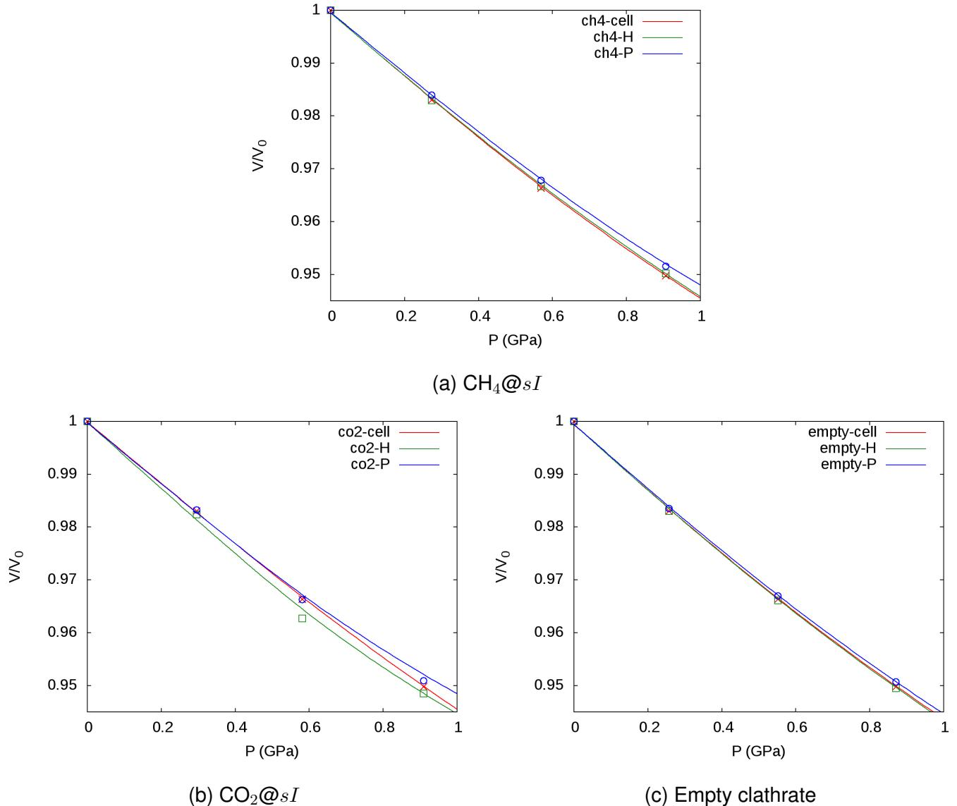
Figure 3.5: Normalized volume-pressure plots for CH<sub>4</sub>@*sI*, CO<sub>2</sub>@*sI* and empty clathrates
