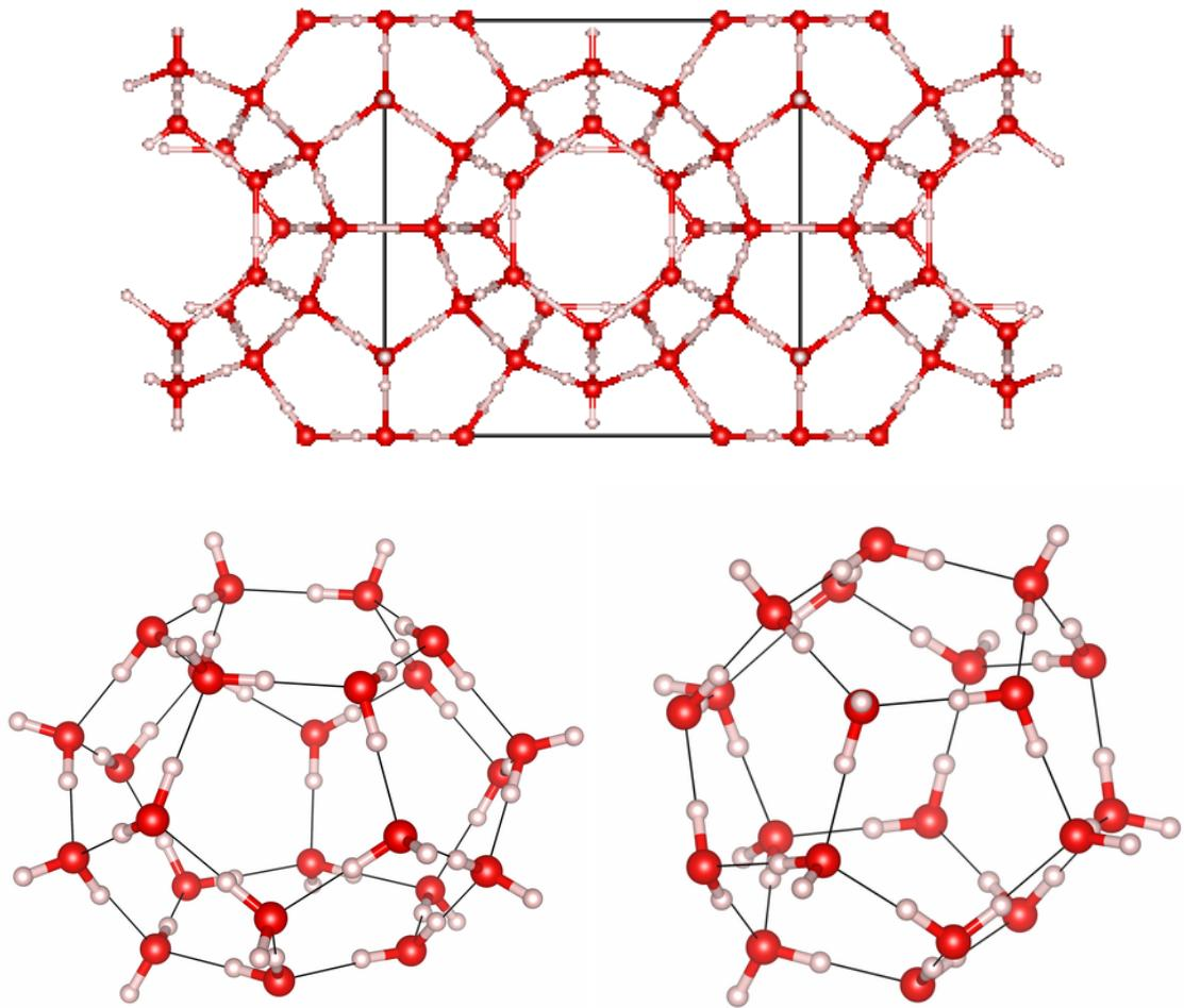
Figure 2.3: Crystalline structure of clathrate *sI* (top), H (left) and P (right) cages
