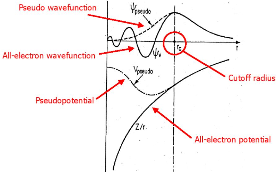
Figure 2.5: Comparison of a pseudopotential with a real potential and its wavefunctions
