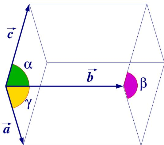
Figure 2.2: Cell parameters and relationship between edges and angles
