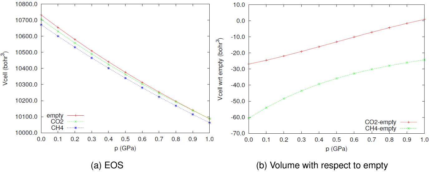
Figure 3.4: EOS curves for  $\text{CH}_4@sI$ ,  $\text{CO}_2@sI$  and empty clathrates (left) and effect of pressure on the unit cell volumes of  $\text{CH}_4@sI$  and  $\text{CO}_2@sI$  with respect to the empty hydrate
