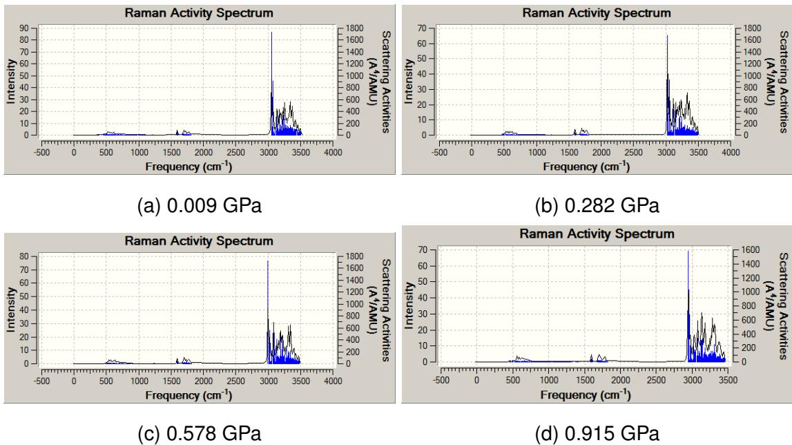
Figure 3.13: Computed Raman spectra of  $\text{CH}_4@sI$
