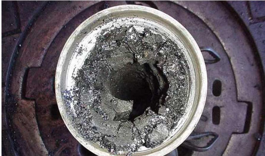
*Figure 7 : Asphaltene deposits inside the pipes[18].*
