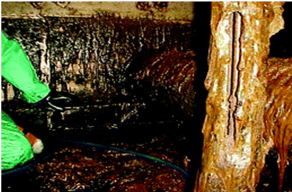
*Figure 8 : Calcium naphthenate deposits in crude oil processing equipment[19].*
