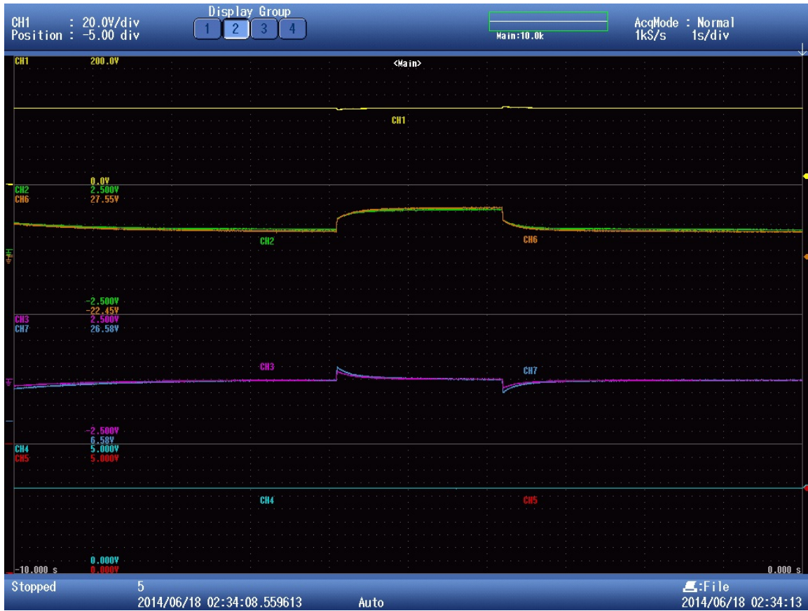
Figure A-4: Experiments results at K = 0.5 and f_{lpf} = 10 Hz: a. DC bus voltage. b. VRFB current. c. LI-IB current. d. Virtual VRFB voltage. e. Virtual LI-IB voltage.
