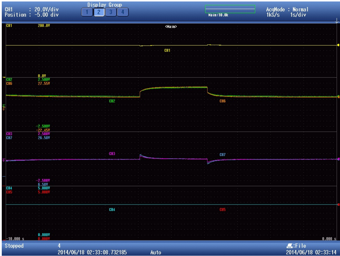
Figure A-3: Experiments results at K = 0.7 and f_{lpf} = 10 Hz: a. DC bus voltage. b. VRFB current. c. LI-IB current. d. Virtual VRFB voltage. e. Virtual LI-IB voltage.
