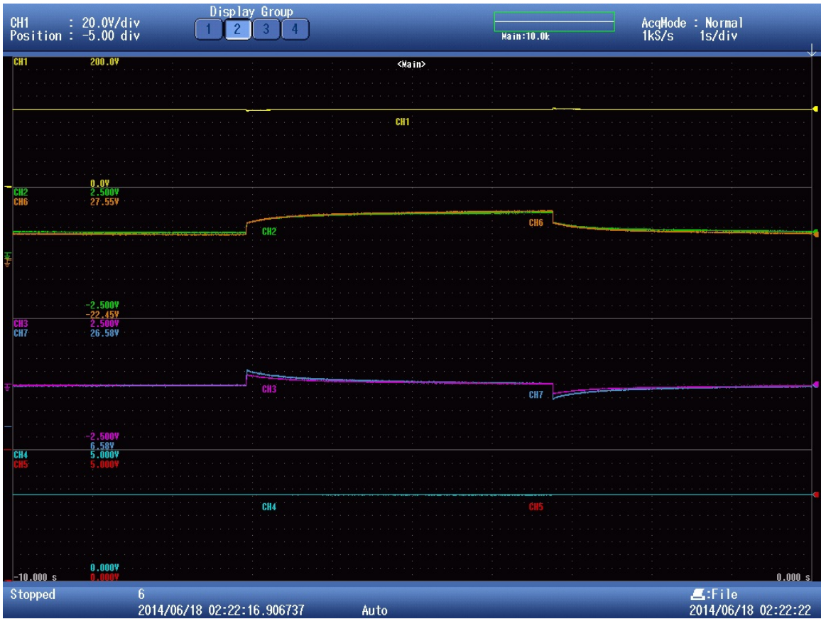
Figure A-6: Experiments results at K = 0.3 and f_{lpf} = 5 Hz: a. DC bus Voltage. b. VRFB current. c. LI-IB current. d. Virtual VRFB voltage. e. Virtual LI-IB voltage.
