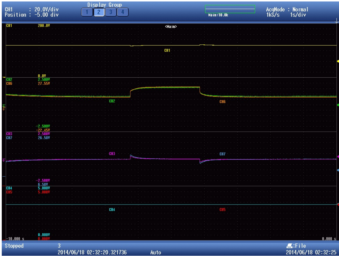
Figure A-2: Experiments results at K = 1.0 and f_{lpf} = 10 Hz: a. DC bus voltage. b. VRFB current. c. LI-IB current. d. Virtual VRFB voltage. e. Virtual LI-IB voltage.
