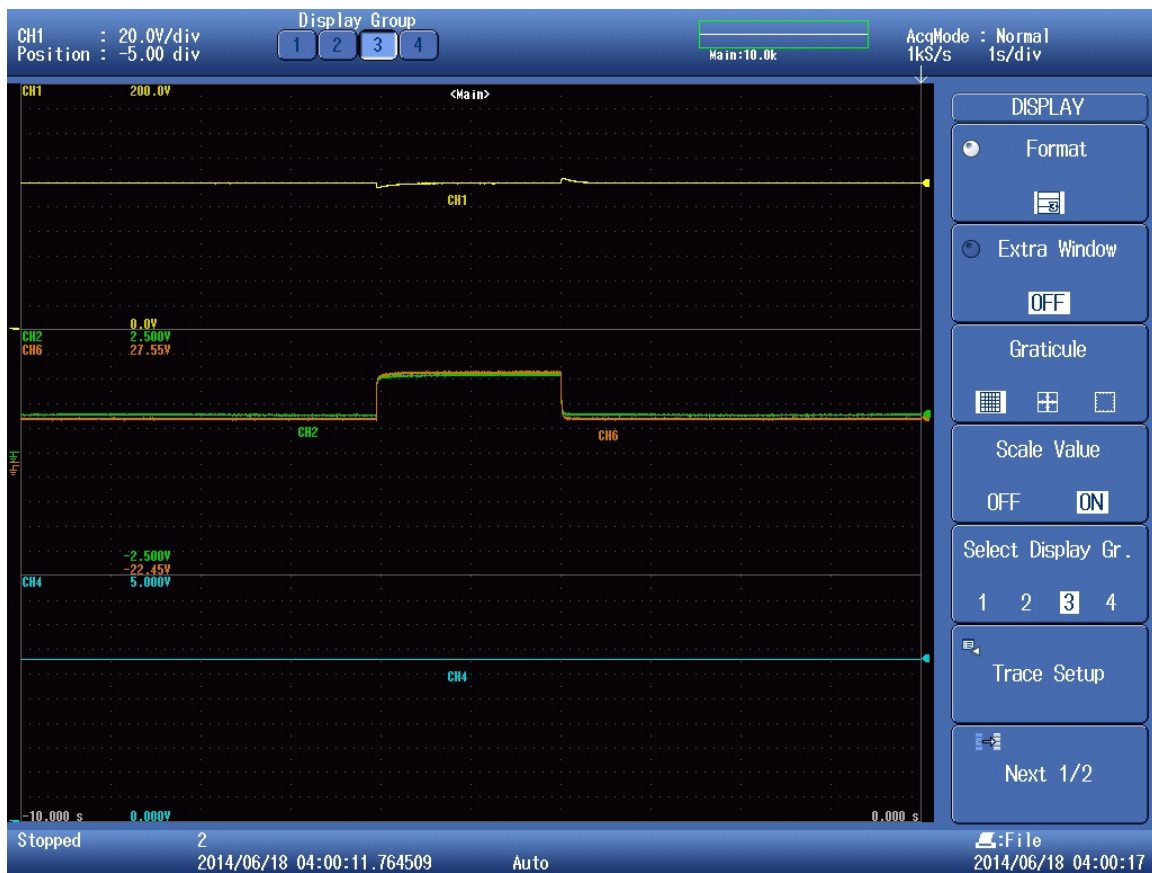
Figure A-1: Experiments results without LI-IB: a. DC bus voltage. b. VRFB current. c. Virtual VRFB voltage.
