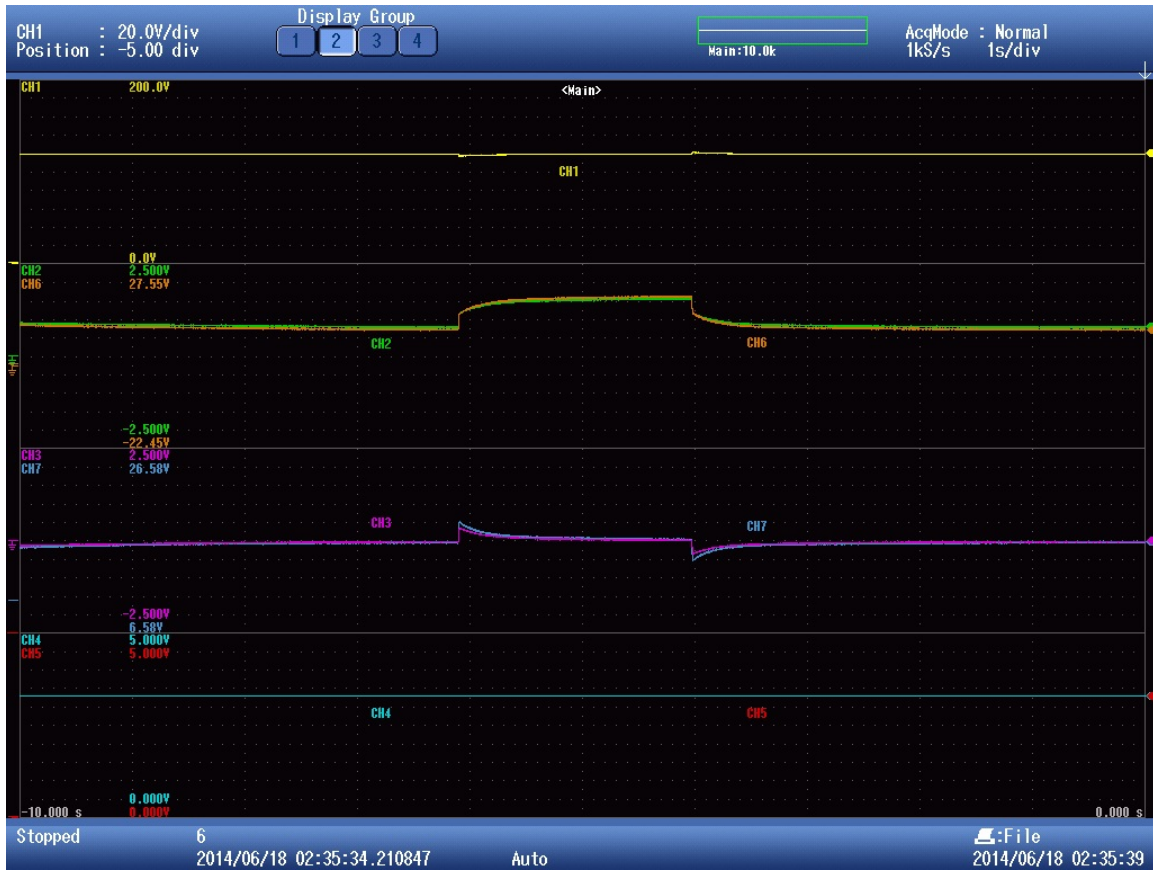
Figure A-5: Experiments results at K = 0.3 and f_{lpf} = 10 Hz: a. DC bus Voltage. b. VRFB current. c. LI-IB current. d. Virtual VRFB voltage. e. Virtual LI-IB voltage.
