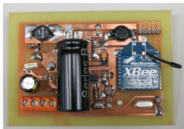
Figure 3. Supply system from PV panel to obtain the 3.3 V and the communication circuitry.
