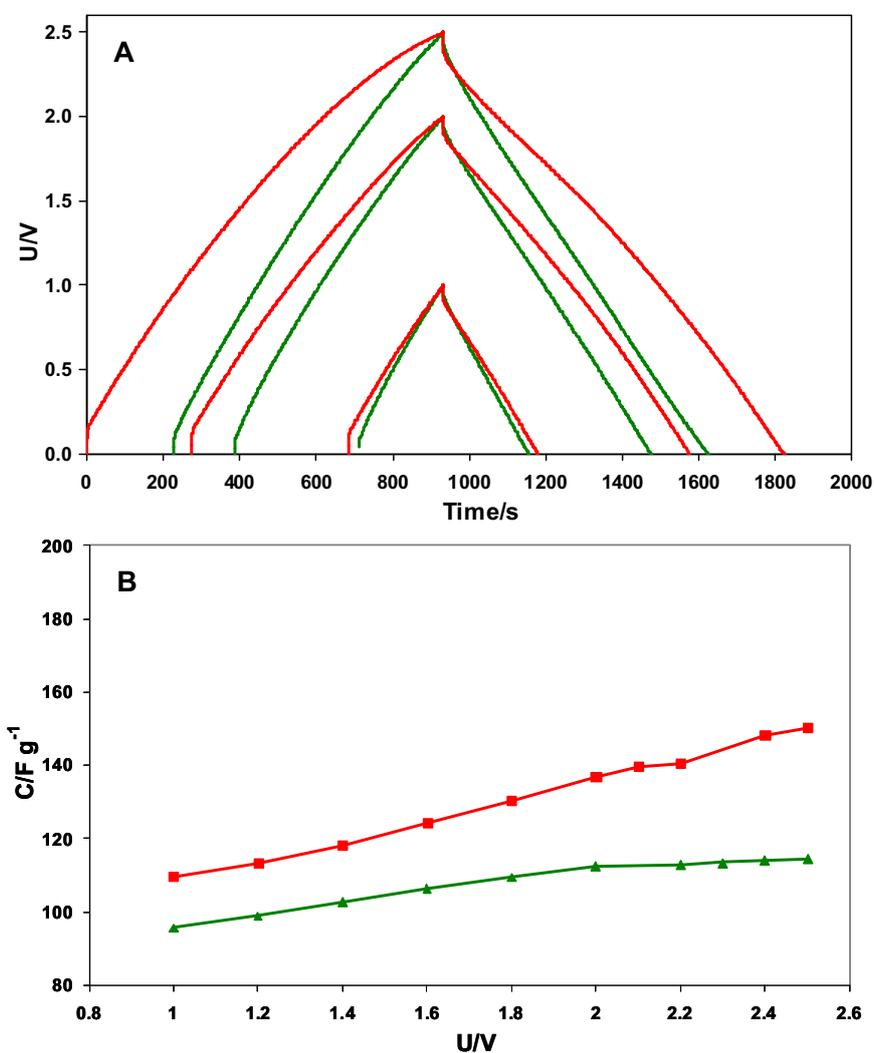
Fig. 8. Galvanostatic characteristics ( $j = \pm 200 \text{ mA g}^{-1}$ ) obtained at different maximum voltages (A) and specific capacitance versus maximum voltage (B) recorded with symmetric 2-electrode cells built in  $\text{NEt}_3\text{H TFSI 200}$  ppm water with AOX (red) or MWV (green).
