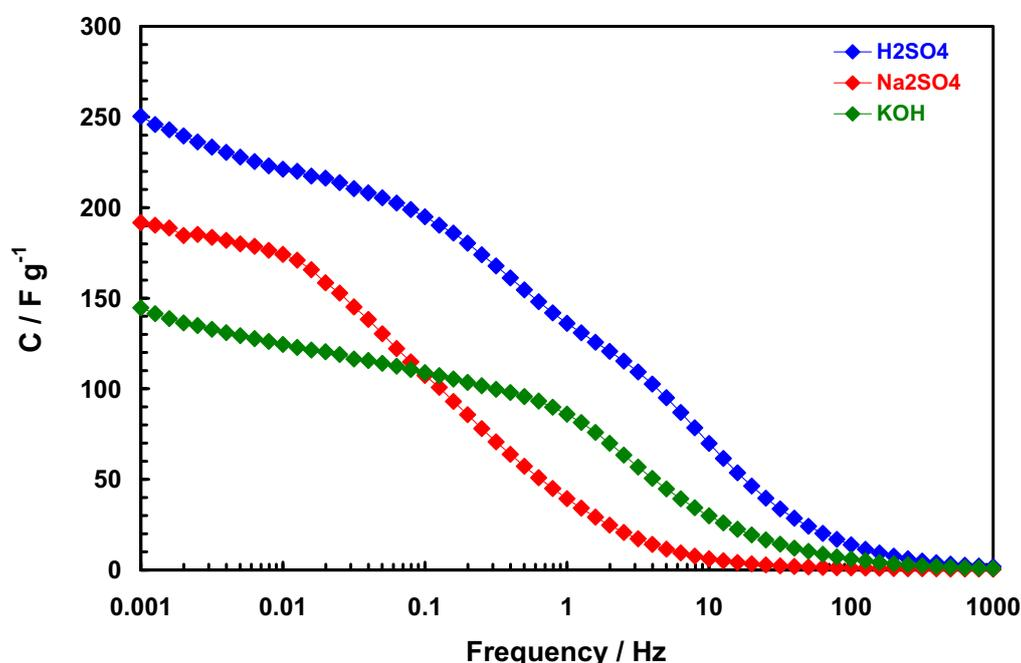
Figure 7. Gravimetric capacitance ( $\text{F g}^{-1}$ ) as a function of the frequency (Hz) for the supercapacitors assembled with the three aqueous solutions studied.
