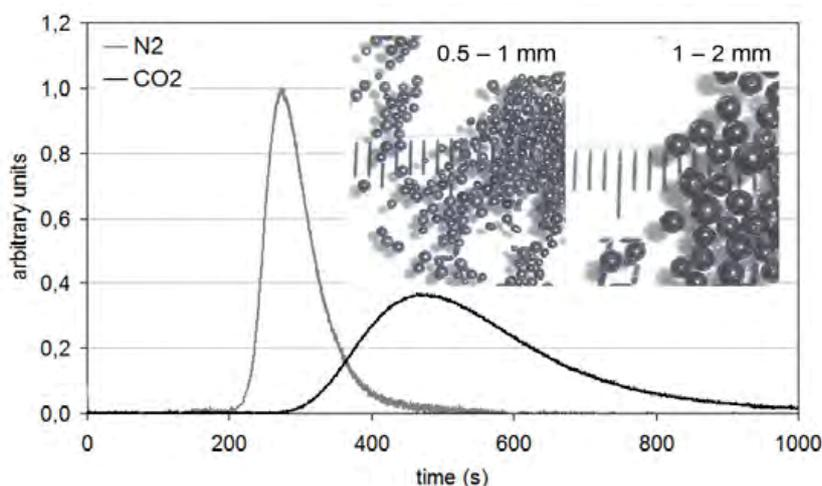
Fig. 14. Carbon xerogel spheres and their potential as fillers for gas separation systems.
