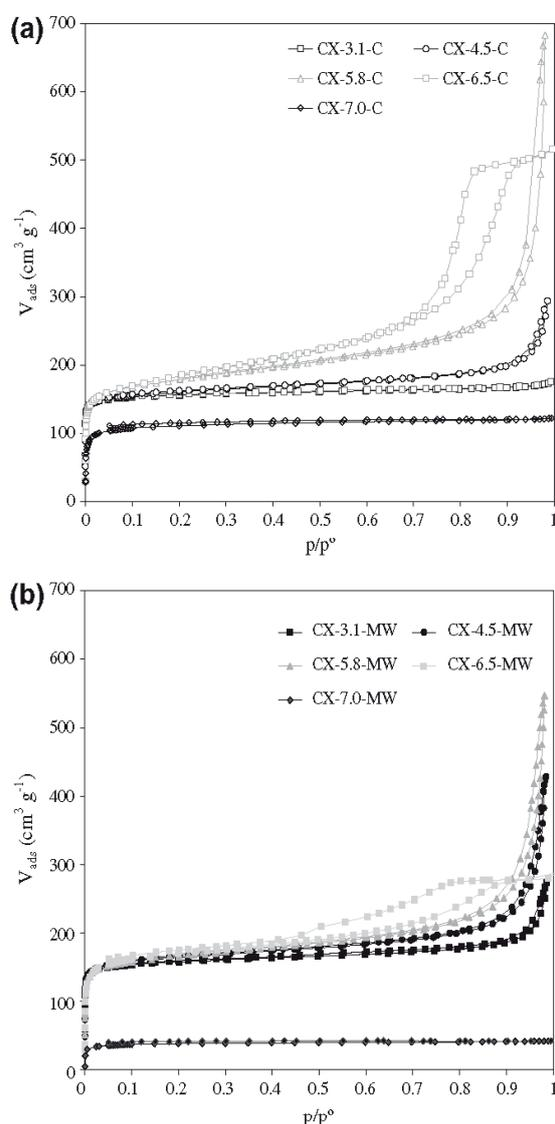
Fig. 2.  $N_2$  adsorption–desorption isotherms of the carbon xerogels studied in this work.
