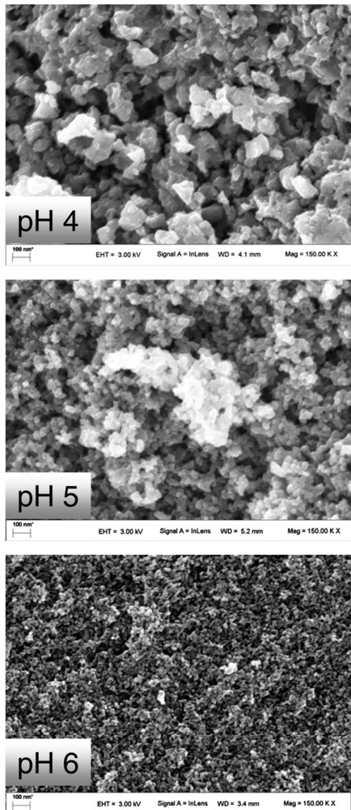
**Fig. 1 – FESEM photographs showing the influence of the pH of the precursor solution on the structure of the carbon xerogel (scale bar = 100 nm).**
