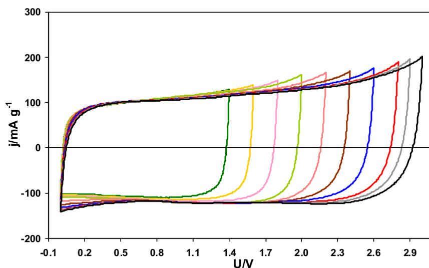
Fig. 7. Cyclic voltammograms obtained in a symmetric 2-electrode cell built using  $\text{NEt}_3\text{H TFSI}$  200 ppm water and MWV as active material.
