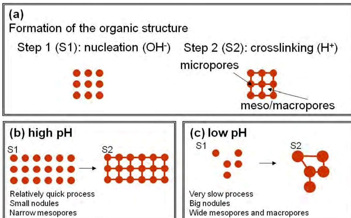
Fig. 5. Schematic representation of the influence of the pH of the precursor solution on the final nanostructure of the carbon gels obtained.
