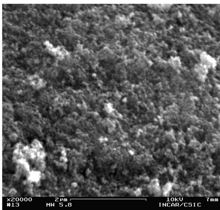
Fig. 12. SEM image of resorcinol-formaldehyde carbon xerogel synthesised in a microwave oven using a precursor solution with a pH of 5.8.
