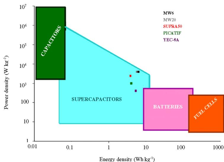
Fig. 6. Ragone plots for supercapacitors assembled with carbon xerogels MW6 and MW20 and the other commercial activated carbons.
