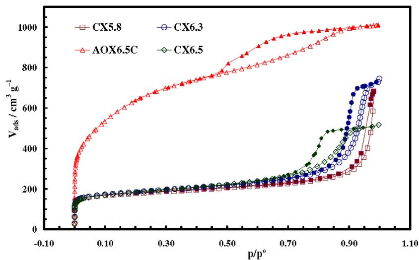
**Figure 1.** Nitrogen adsorption (open symbol)/desorption (filled symbol) isotherms for synthesized carbon xerogels
