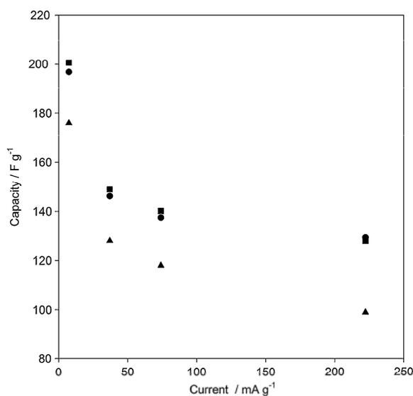
**Fig. 5** Rate capability results for E18 (filled circles), E9 (filled squares), and E0 (filled triangles). Charge current, 7.4 mA g<sup>-1</sup>
