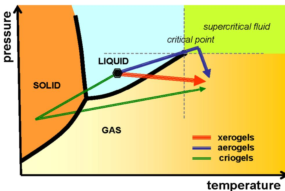
Fig. 6. Scheme of the different ways of removing the solvent used in the synthesis of organic gels.
