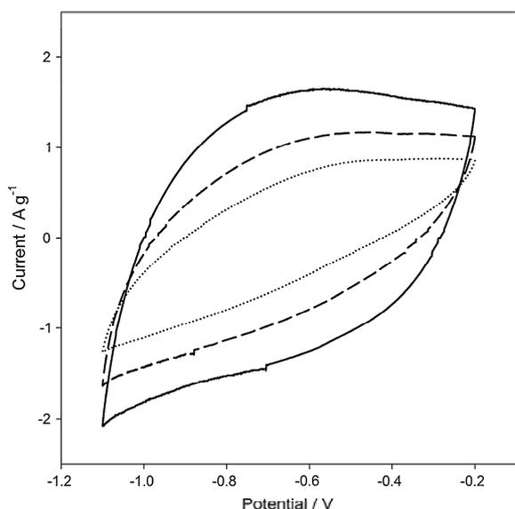
**Fig. 4** Voltammograms of: **a** E0 (dotted line), **b** E9 (dashed line), and **c** E18 (solid line).  $E_{\text{sa}} = -0.20$  V,  $E_{\text{sc}} = -1.10$  V,  $\nu = 1.10^{-2}$  V s<sup>-1</sup>, 6 M KOH;  $T = 303$  K
