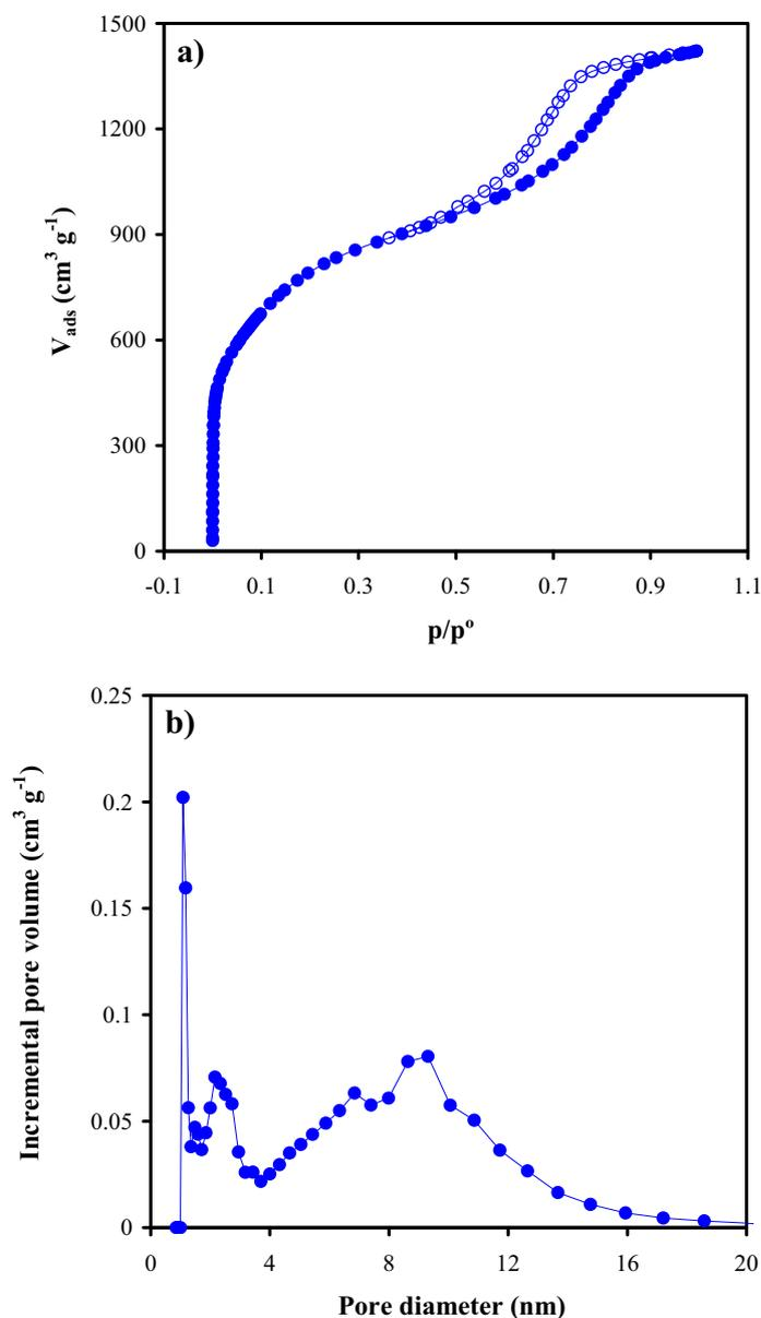
Figure 1.  $N_2$  adsorption-desorption isotherm (a) and pore size distribution (b) for the activated carbon xerogel used as electrode material.
