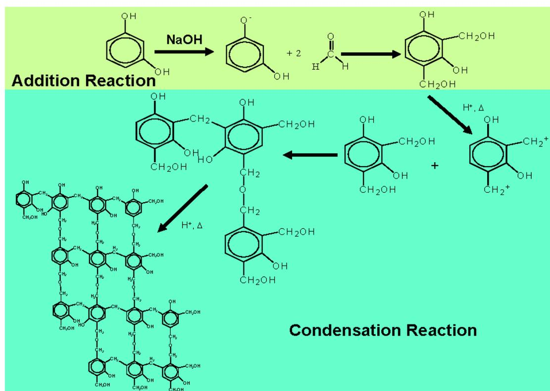
Fig. 4. Mechanism of resorcinol-formaldehyde polymerization (based on reference Al-Mutasheb & Ritter, 2003).
