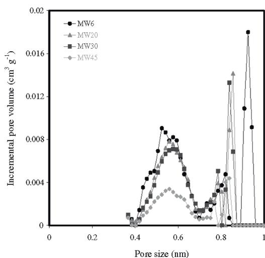
Fig. 3. Pore size distribution of carbon xerogels synthesized, obtained by applying the DFT method to  $\text{CO}_2$  adsorption isotherms at 273 K.
