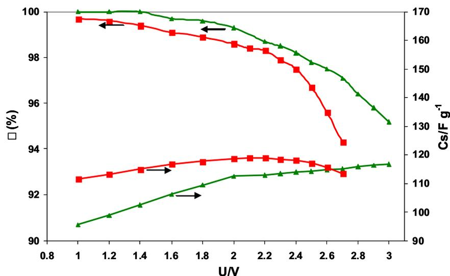
Fig. 10. Efficiency and specific capacitance at various maximum voltages recorded for symmetric 2-electrode cells with MWV as active material. Effect of the nature of the electrolyte: NEt<sub>3</sub>H TFSI (green) or NEt<sub>3</sub>H TFSI/PC (1:1) (red).
