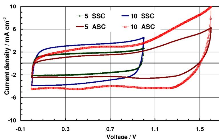
**Figure 7.** Comparison of the voltammograms of carbon xerogels-based supercapacitors in symmetric (SSC) and asymmetric (ASC) configurations. Voltage sweep rates: 5 and 10  $\text{mVs}^{-1}$ . Cell voltage window from 0 to 1 V for SSC and from 0 to 1.6 V for ASC.
