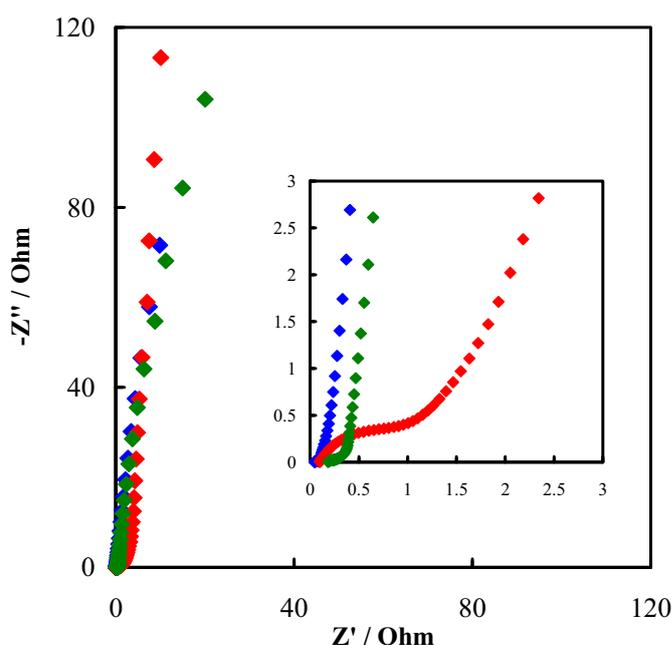
Figure 6. Nyquist plots for 4  $\text{cm}^2$  two-electrode cells and three different aqueous electrolytes. The insert shows the high frequency region of impedance.
