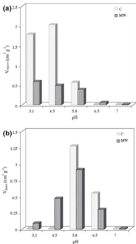
Fig. 4. Macropore and mesopore volume of the carbon xerogels synthesized in this work.
