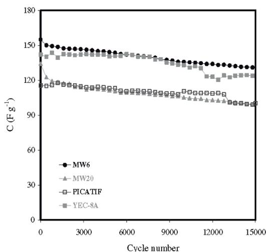
Fig. 7. Evolution of specific capacitance ( $F g^{-1}$ ) with the number of galvanostatic cycles for two carbon xerogels synthesized in this work and two commercial activated carbons ( $U = 1.0 V$ ;  $i = 500 mA g^{-1}$ ).
