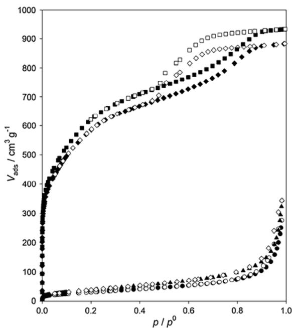
**Fig. 3** Adsorption–desorption isotherms of  $N_2$  at  $-196$  °C for: **a** MWCNT (*filled triangles*), **b** MWCNTt (*filled circles*), **c** AOX (*filled squares*), and **d** AOXt (*filled diamonds*)
