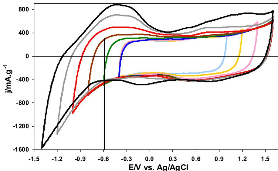
Fig. 5. 3-electrode cyclic voltammograms of MWV recorded in  $\text{NEt}_3\text{H TFSI}$  with 5000 ppm water; scan rate  $2 \text{ mV s}^{-1}$ .
