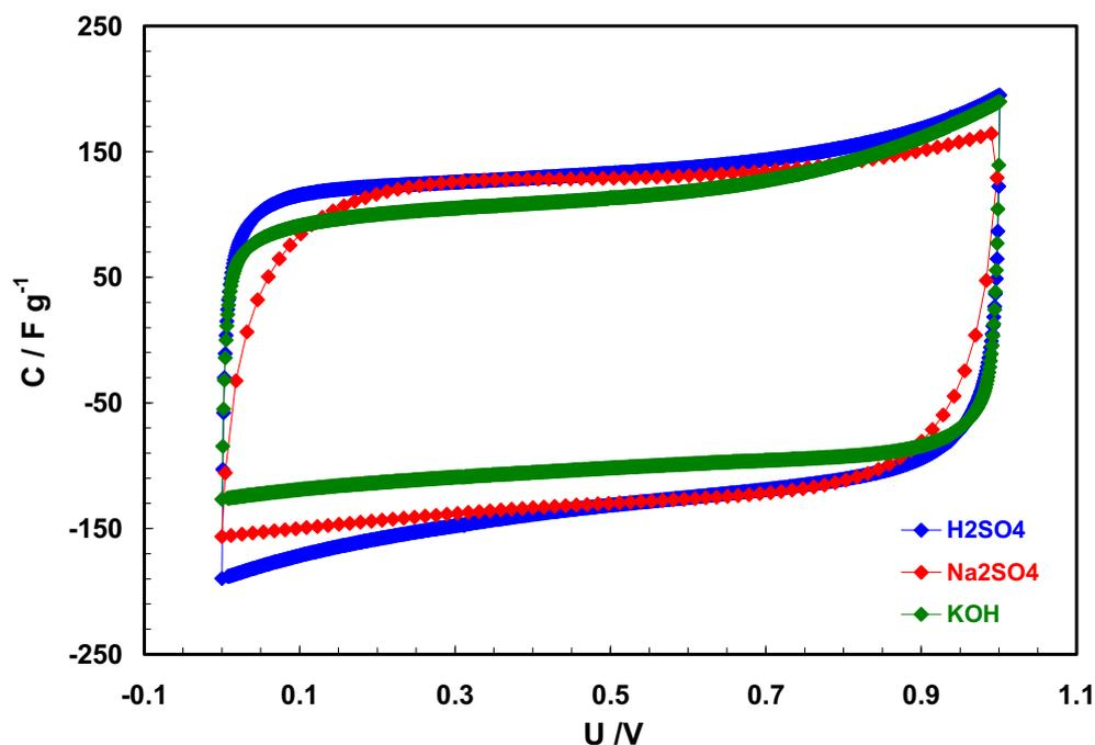
Figure 5. Cyclic voltammograms obtained in 2-electrodes cells ( $4 \text{ cm}^2$ ) and three electrolytes with different pH ( $\text{H}_2\text{SO}_4$ ,  $\text{Na}_2\text{SO}_4$  and  $\text{KOH}$ ).
