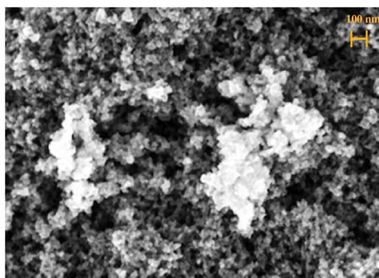
Fig. 2. SEM image of carbon xerogel chemically activated for 6 min (MW6).
