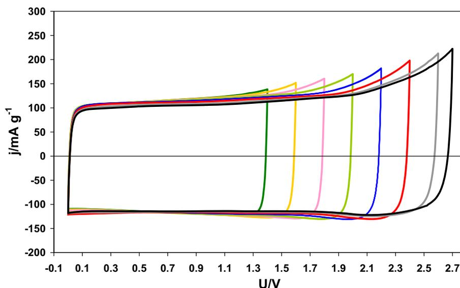
Fig. 9. Cyclic voltammograms obtained in a symmetric 2-electrode cell built using  $\text{NEt}_3\text{H TFSI / PC}$  with MWV as active material.
