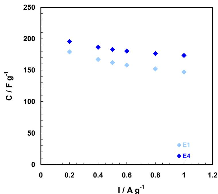
Figure 4. Variation of specific capacitance ( $\text{F g}^{-1}$ ) with current density for cells built with 1 and 4  $\text{cm}^2$  electrodes and  $\text{H}_2\text{SO}_4$  1M as electrolyte (maximum voltage = 1.0 V).
