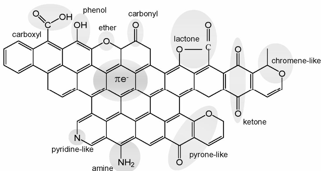
Fig. 7. Main functionality groups that can be incorporated into carbon gels by post-synthesis treatments.
