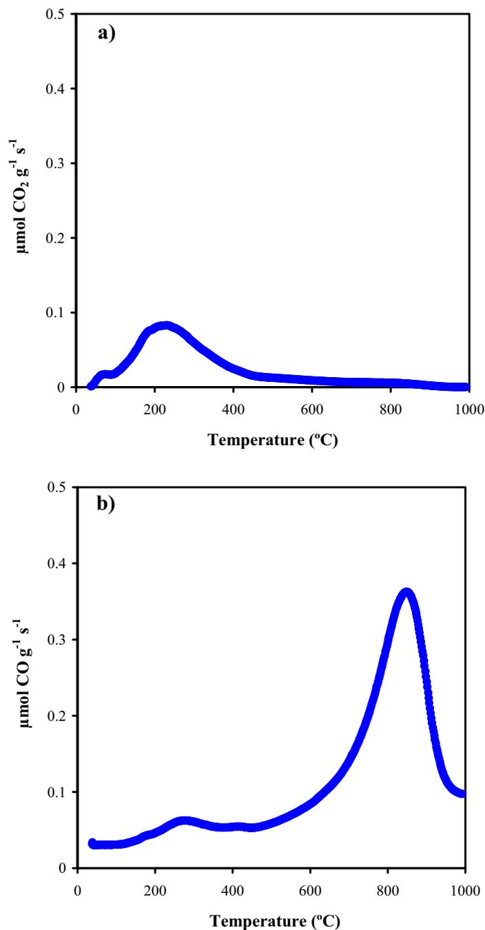
Figure 2. CO<sub>2</sub> (a) and CO (b) profiles obtained by TPD experiments for ACX sample.
