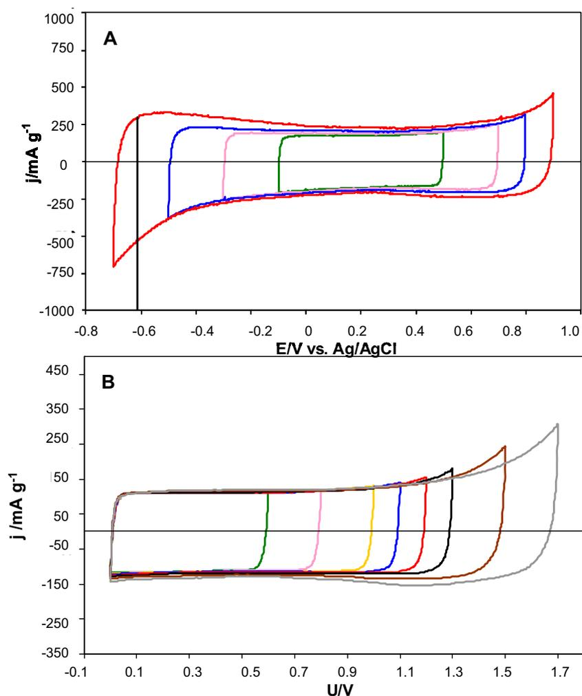
Fig. 3. 3-electrode (A) and 2-electrode (B) cyclic voltammograms of AOX in  $\text{PyNO}_3$  with 1110 ppm water; scan rate  $2 \text{ mV s}^{-1}$ .
