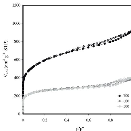
Fig. 4.  $\text{N}_2$  adsorption-desorption isotherms of samples treated at different activation temperature (700, 600 and 500 °C).
