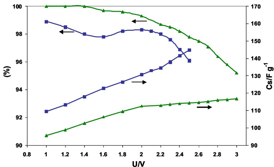
Fig. 6. Efficiency and specific capacitance at various maximum voltages recorded for symmetric 2-electrode cells with MWV as active material and  $\text{NEt}_3\text{H TFSI}$  as electrolyte. Effect of water content: 200 ppm (green) or 5000 ppm (blue).
