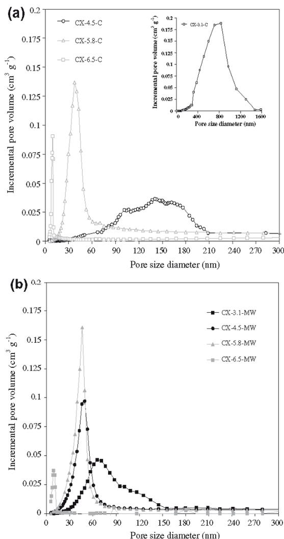
Fig. 3. Pore size distribution of carbon xerogels prepared with different initial pHs and heating methods: conventional (a) and microwave radiation (b).
