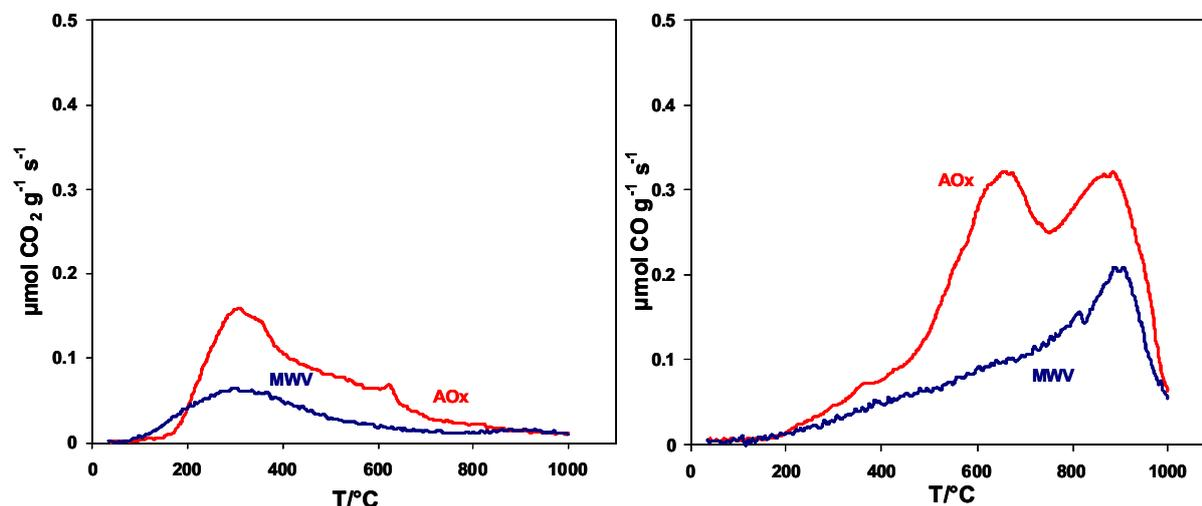
Fig. 1.  $\text{CO}_2$  (A) and  $\text{CO}$  (B) profiles obtained by TPD experiments with AOX and MWV samples.
