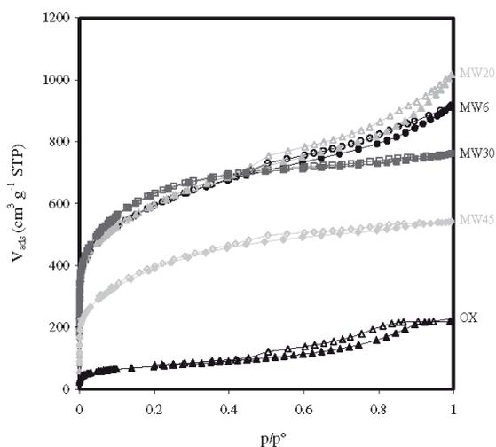
Fig. 1. N<sub>2</sub> adsorption–desorption isotherms of carbon xerogels obtained from different activation times.
