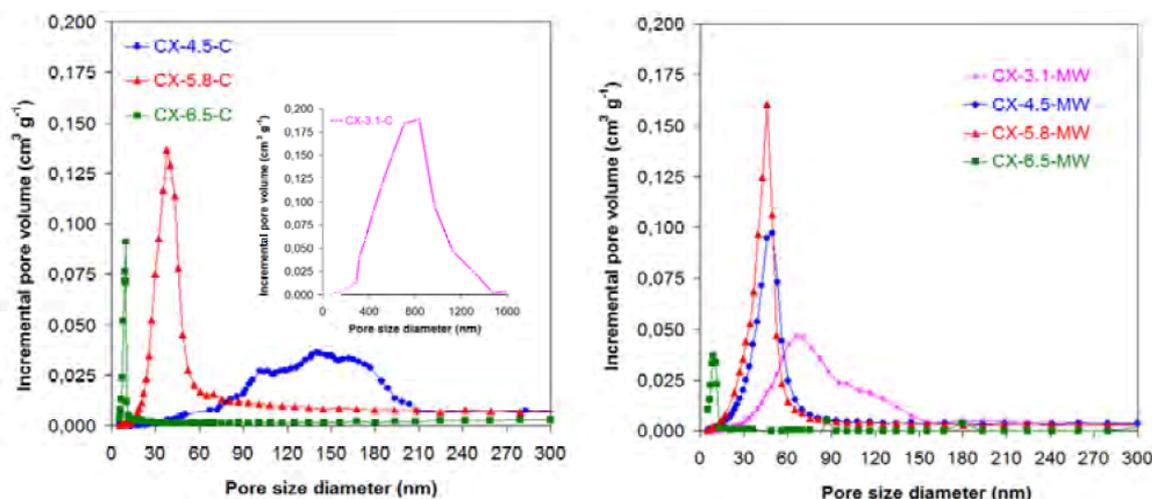
Fig. 10. Pore size distribution of resorcinol-formaldehyde prepared with different pH and heating mechanisms: conventional (a) and microwave radiation (b) (adapted from reference Calvo et al., 2011a).
