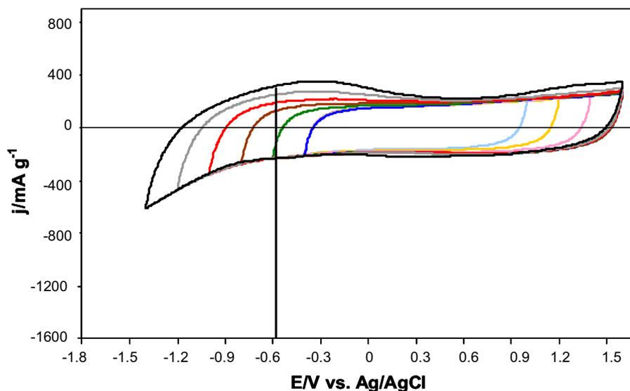
Fig. 4. 3-electrode cyclic voltammograms of MWV with  $\text{NEt}_3\text{H}$  TFSI (200 ppm water); scan rate  $2 \text{ mV s}^{-1}$ .
