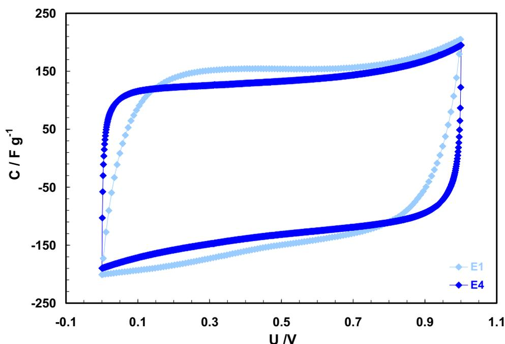
Figure 3. Cyclic voltammograms for supercapacitors using  $\text{H}_2\text{SO}_4$  1.0 M as electrolyte and carbon xerogel-based electrodes of different size (scan rate =  $10 \text{ mV s}^{-1}$ ).
