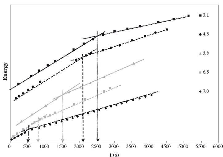
**Fig. 1.** Representation of the gelation point of several RF xerogels obtained by microwave heating from precursor solutions with different pHs. For a better visualization of the gelation point (i.e. time at which the change in the slope takes place) energy values were displaced along the y-axis by adding a constant to the actual values. For that reason no scale is shown in the y-axis.
