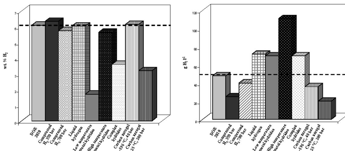
Fig. 13. Gravimetric and volumetric storage capacity of several hydrogen storage systems
