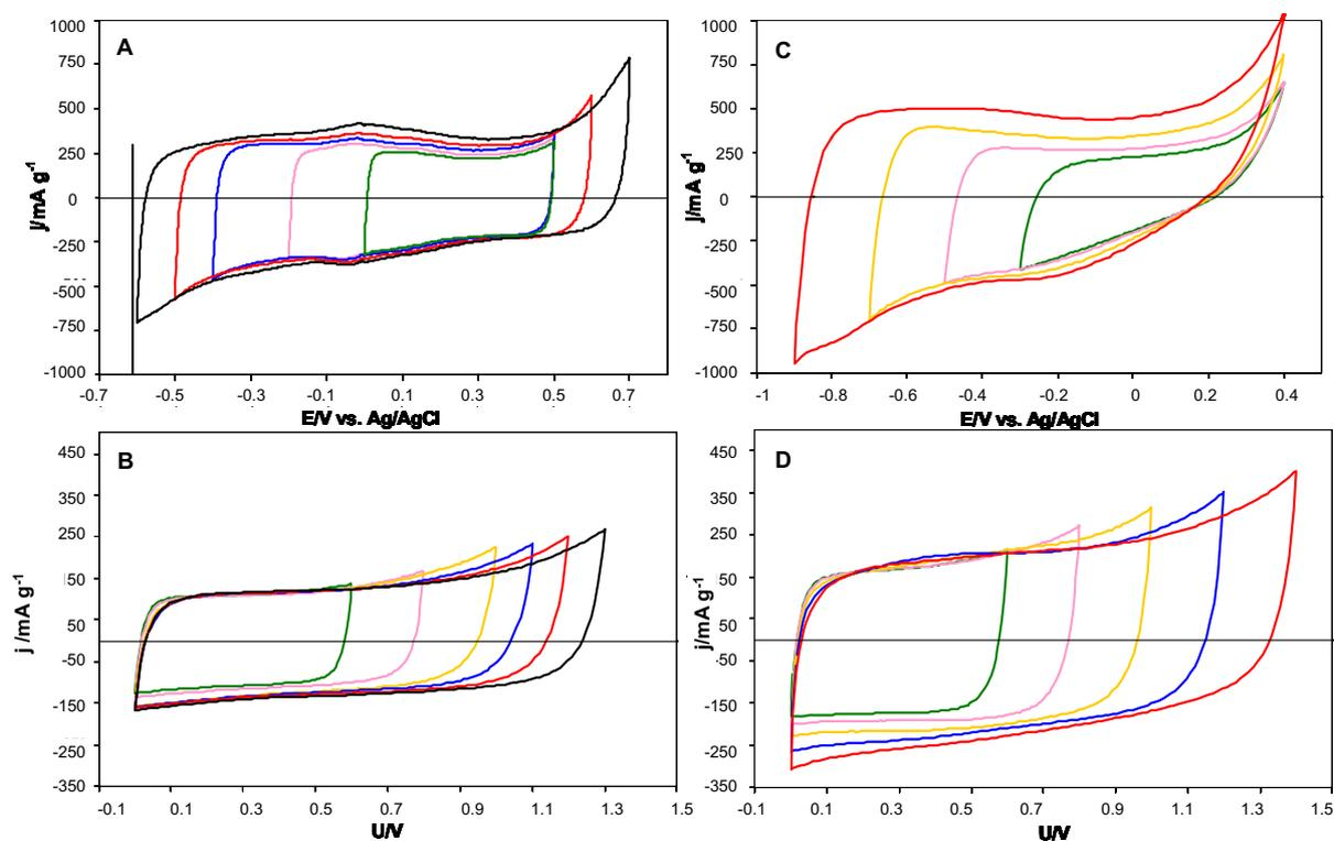
Fig. 2. 3-electrode (A) and 2-electrode (B) cyclic voltammograms of AOX in PyNO<sub>3</sub>-pH7 and PyNO<sub>3</sub>-pH 11 (C and D); scan rate 2 mV s<sup>-1</sup>.
