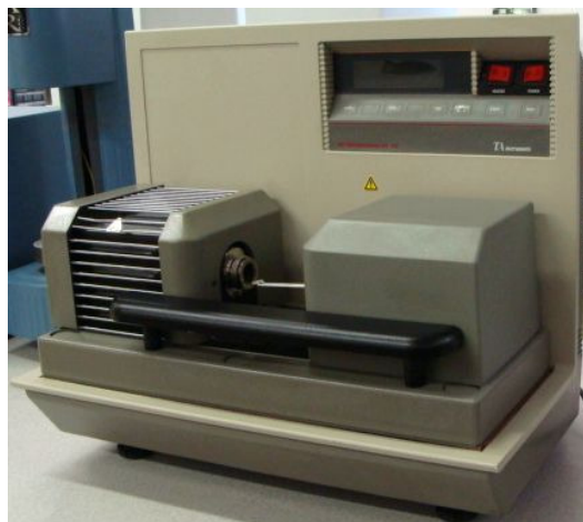
Figura 3.3. Termobalanza TA Instruments STD 2960
