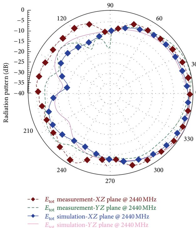
FIGURE 21: Simulated and measured radiation patterns (total E-field for the XZ and YZ planes) for the proposed dual-band L-shape PIFA at 2440 MHz (central frequency for the IEEE 802.11b,g band).
