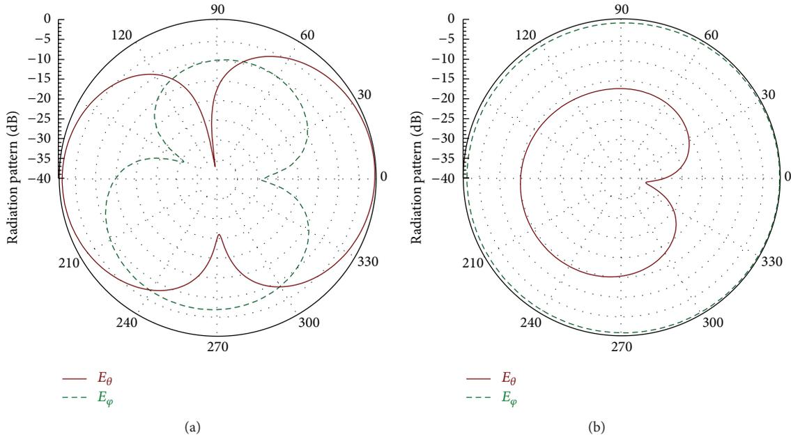
FIGURE 17: Simulated radiation patterns ( $E_\theta$  and  $E_\phi$  components normalized to the electric field amplitude at  $\theta = 0$ ) for the proposed dual-band L-shape PIFA at 670 MHz: (a)  $\phi = 45^\circ$  plane; (b)  $\phi = -45^\circ$  plane.
