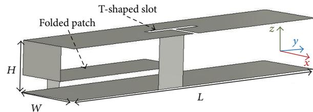
FIGURE 5: The inclusion of a T-shaped slot as well as a folded patch results in a wide impedance bandwidth in the PIFA presented in [15].
