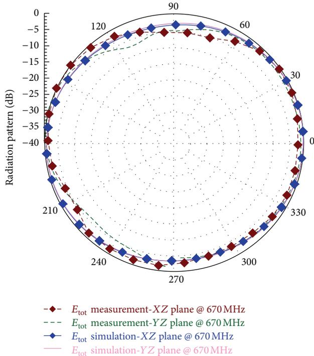
FIGURE 20: Simulated and measured radiation patterns (total E-field for the XZ and YZ planes) for the proposed dual-band L-shape PIFA at 670 MHz (central frequency for the DVB-T band).
