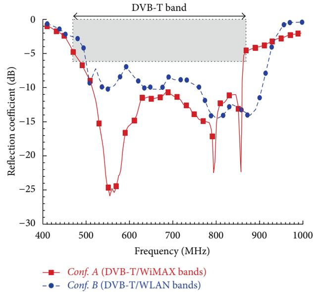
FIGURE 9: Measured reflection coefficient for the two PIFAs in [16, 18], in the DVB-T band.
