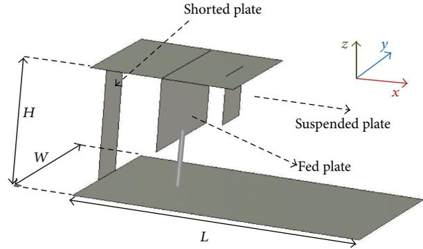
FIGURE 3: A PIFA consisting of a planar rectangular monopole top-loaded with a rectangular patch attached to two rectangular plates, one is shorted to the ground and the other is suspended [13].
