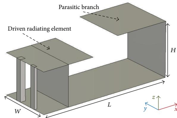
FIGURE 6: A PIFA characterized by a driven (fed) radiating element separated by a small gap from a parasitic branch [16].
