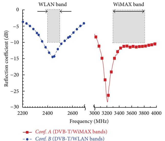
FIGURE 10: Measured reflection coefficient for the two PIFAs in [16, 18], in the WiMAX and WLAN bands, respectively.
