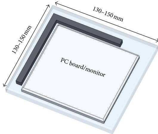
FIGURE 11: Example of a 3D view of a typical monitor chassis. The available space for the antenna is dark highlighted.
