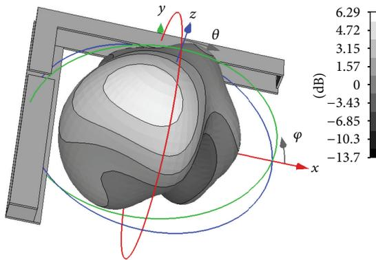
FIGURE 16: Simulated 3D antenna gain (dBi) for the dual-band L-shape PIFA at 2440 MHz.
