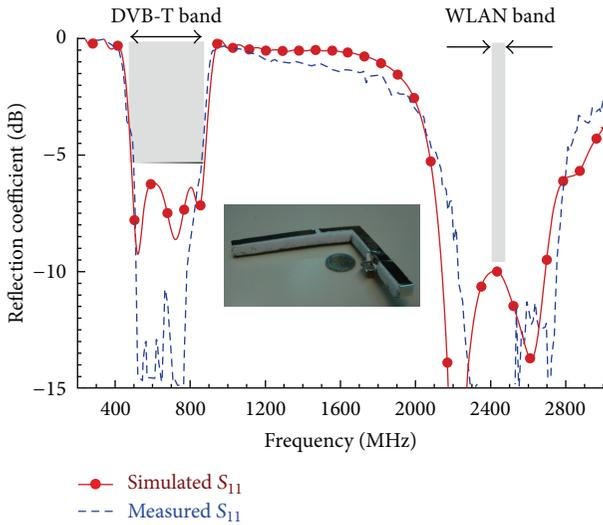
FIGURE 18: Simulated and measured reflection coefficient for the proposed dual-band L-shape PIFA.
