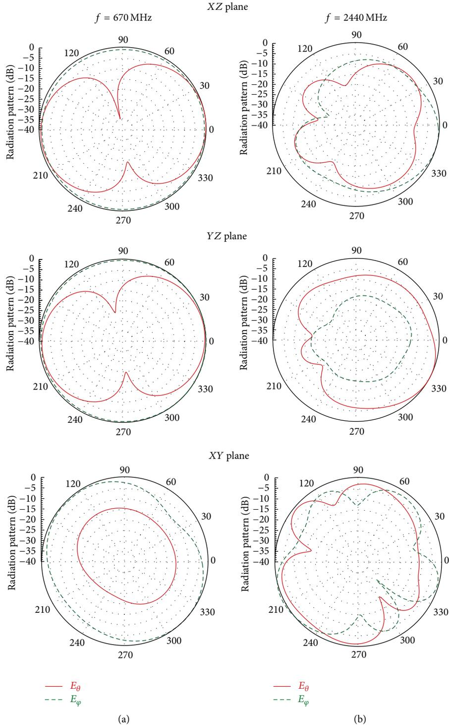
FIGURE 14: Simulated radiation patterns ( $E_\theta$  and  $E_\phi$  components normalized to the electric field amplitude at  $\theta = 0$ ) for the proposed dual-band L-shape PIFA: (a) 670 MHz (central frequency for the DVB-T band); (b) 2440 MHz (central frequency for the IEEE 802.11b,g band).
