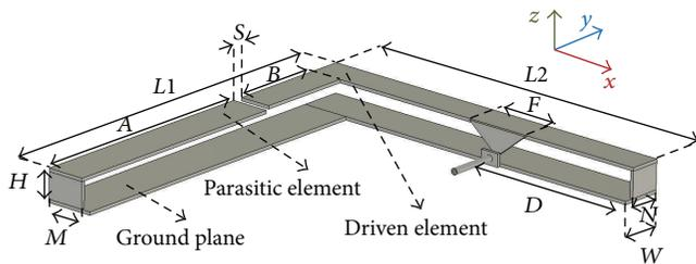
FIGURE 12: Geometry of the proposed dual-band L-shape PIFA.
