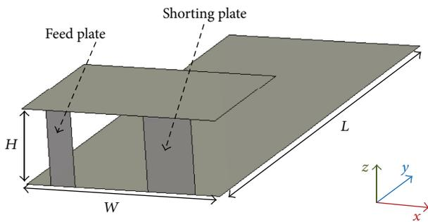
FIGURE 2: A PIFA where bandwidth enlargement can be achieved by optimizing the widths of the feeding and shorting plates [12].
