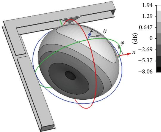
FIGURE 15: Simulated 3D antenna gain (dBi) for the dual-band L-shape PIFA at 670 MHz.
