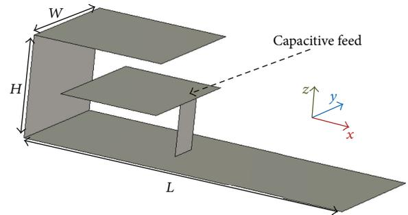
FIGURE 4: A PIFA where a large impedance bandwidth has been obtained by using a capacitive feeding [14].
