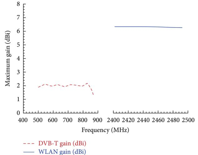
FIGURE 13: Simulated gain for the proposed dual-band L-shape PIFA as a function of frequency.
