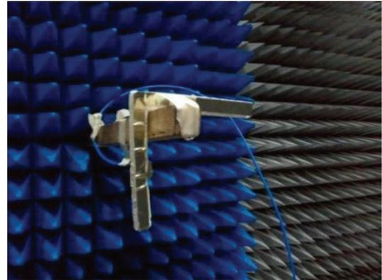
FIGURE 19: Antenna prototype mounted on the rotating platform for radiation pattern measurements.
