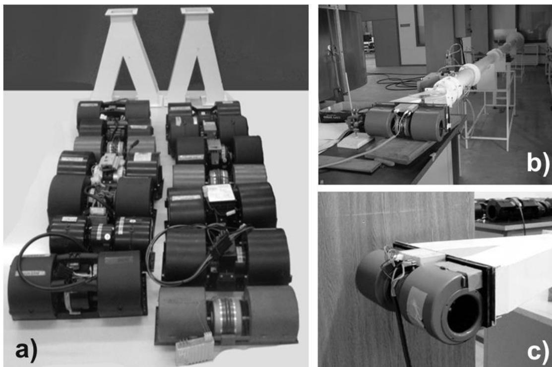
Figure 3: a) Tested fans and Y-shaped ducts. b) Typical arrangement for performance tests. c) Detail of the ventilation unit connected to the Y-shaped duct.
