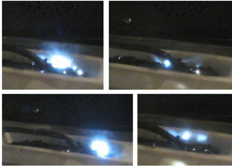
**Fig. 2 – Ball lightning plasma formation at the initial stages of the experiment, (average temperature as measured by a thermocouple: <math><400\text{ }^\circ\text{C}</math>). The experiment was carried out over activated carbon and in the presence of a thermocouple.**
