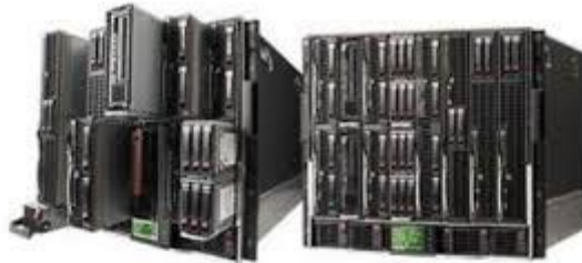
Fig. 6. Blade systems HP C7000 server
