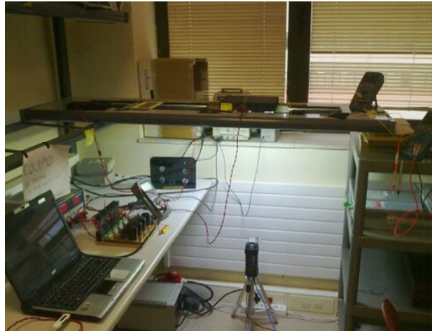
Fig. 2.39. Experimental workbench for measuring the lamp temperature by IR thermography.
