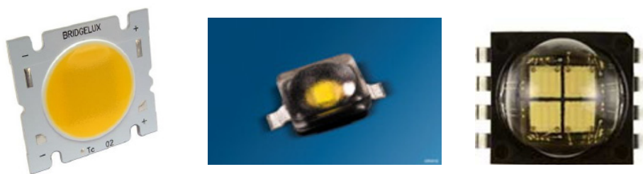
Fig. 1.25. High-Power LEDs. Left: RS Array by Bridgelux. Centre: Diamond Dragon by Osram. Right: XLamp MC-E by Cree.
