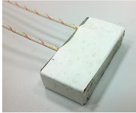
Fig6.13. Thermocouples attached to the magnet
