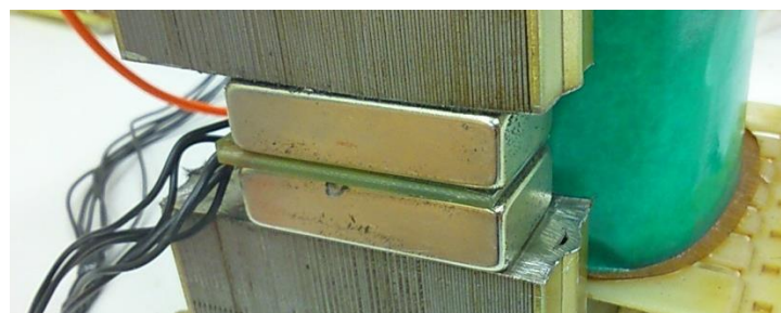
Fig6.15. I2C sensor card between two magnets
