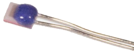
Fig6.2 PT100 thin film package. Source:RS
