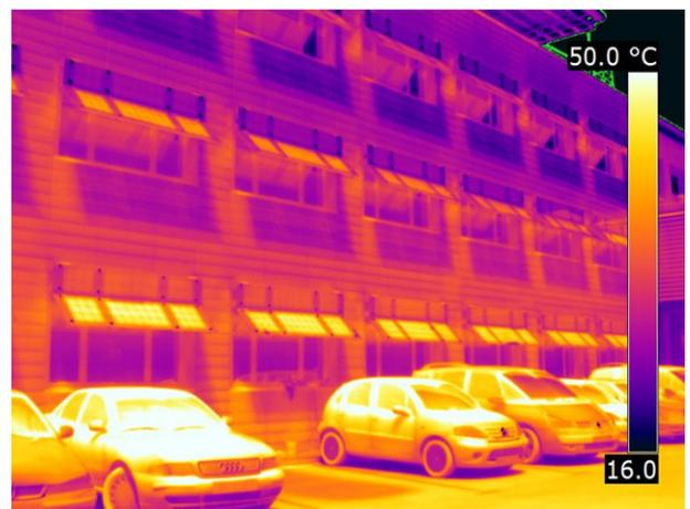
Fig. 8. Thermograph of the south façade of Madrid building, springtime, 14:00 (perpendicular solar radiation  $779 \text{ W/m}^2$ , exterior temperature  $15.6 \text{ }^\circ\text{C}$ ).
