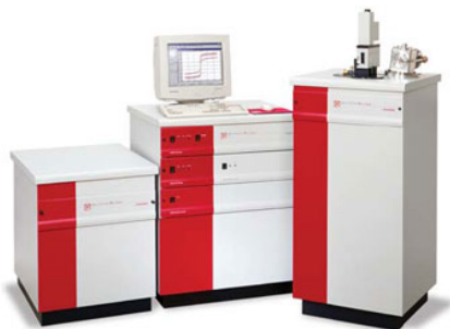
Figure 2.7: Magnetic Property Measurement System XL-5 system at the Institute of experimental physics of the Slovak Academy of Science.
