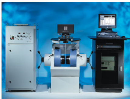
Figure 2.5: Vibrating Sample Magnetometer system at the University of Sevilla.
