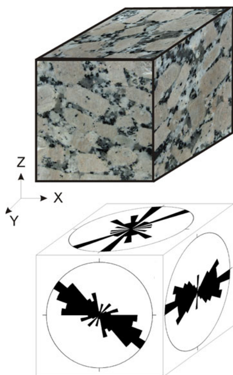
Fig. 7 K-feldspar orientation in R granite. XZ and ZY planes show the most quantity of oriented crystals with 92 and 65 measurements, respectively. In the XY slab, only 18 oriented K-feldspar were found. The slab with the greatest bowing followed the YZ plane and showed K-feldspar parallel to the Y axis
