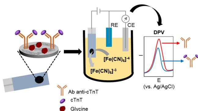
Fig. 6. Scheme of the immunosensor and the electrochemical principle of detection developed by Silva et al. [114].
