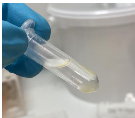
Figure 4.5. Second liquid phasic in the reaction mixture with catalyst.
