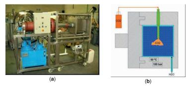
Figure 1. (a) Photogram and diagram of operation of test equipment named ROCKTESTCO2; (b) Description of what is contained in the second panel. Figures should be placed in the main text near to the first time they are cited. A caption on a single line should be centered. Note: please refer to the figure in the main text.
