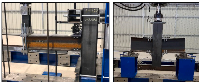
Fig. 2. Type of beam-column joints tested. (a) Beam connection to one side of the column (SMS); (b) Connection with beam on both sides of the column (DMS).
