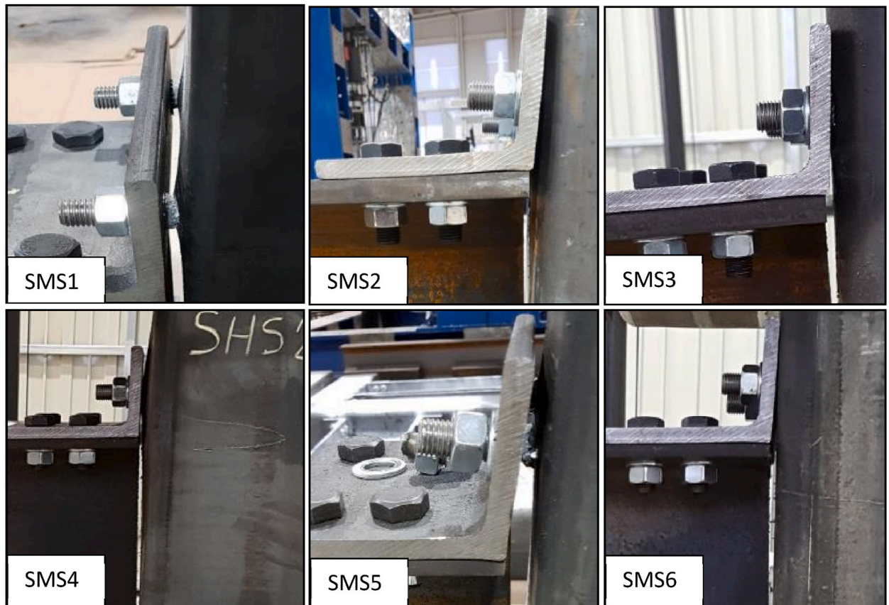
Fig. 11. Deformations observed during the tests for the specimens SMS1 to SMS6.
