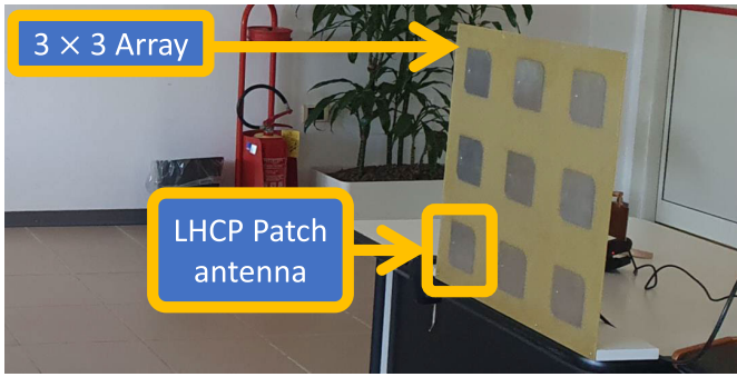
Fig. 3. 3 \times 3 array of LHCP patch antennas used for the measurements. By changing the feeding network, the antenna can radiate either an FF broadside pattern or an NFF spot.
