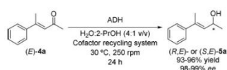
Scheme 3. Screening of ADHs for the bioreduction of ketone ( E )- 4a for the synthesis of ( E )- 5a alcohol enantiomers depending on the ADH of choice.
