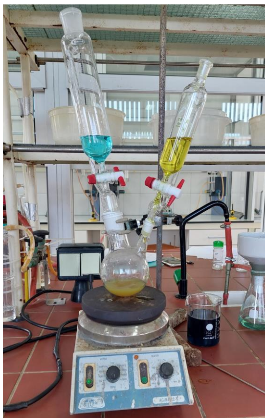
Figure S2. Experimental setup for the synthesis of CuHCF and Prussian Blue (the photo corresponds to the CuHCF example).
