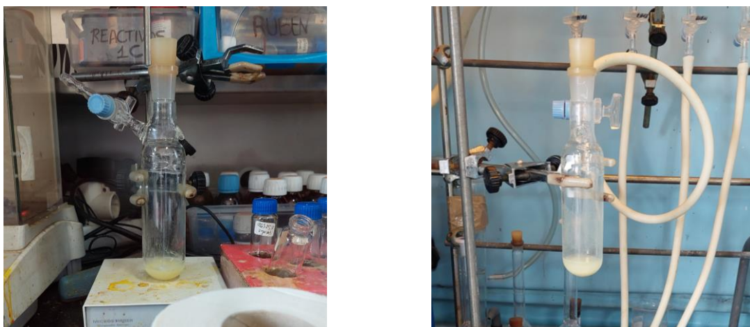
Figure S4. Reaction crude during the synthesis of [\text{PdI}\{(\text{C}_6\text{H}_4)\text{-4-NH}_2\}(\text{PPh}_3)_2] (C) (left) and suspension formed during the washing procedure (right).
