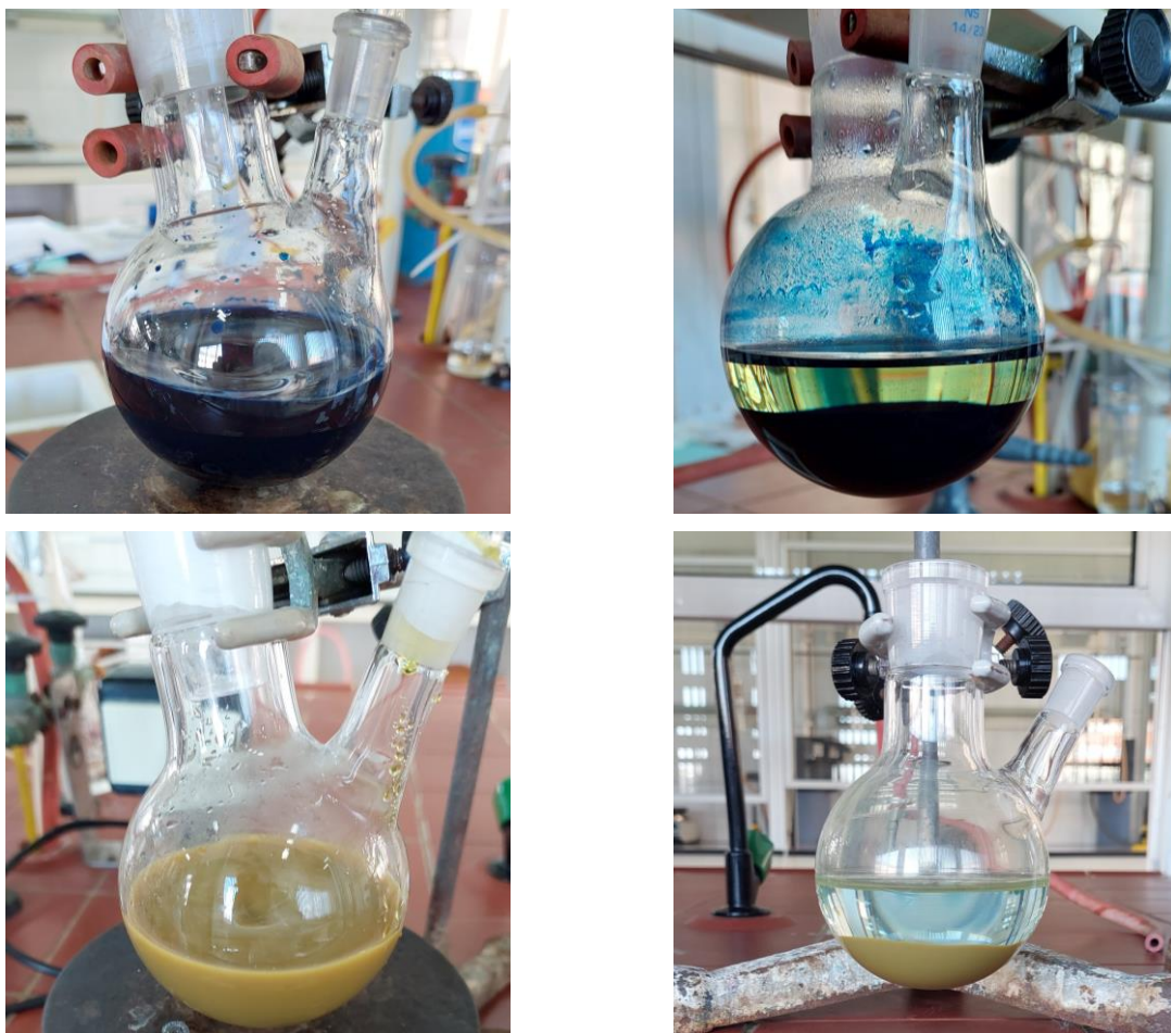
Figure S3. Prussian Blue (PB) (top) and CuHCF (A) (bottom) suspensions before and after leaving them to settle overnight.
