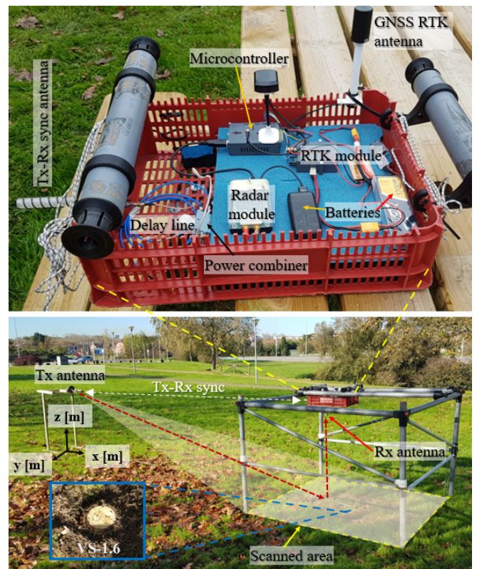
Fig. 8. Picture of the implemented FL-DL-GPR architecture, showing a detail of the Rx payload (upper picture). Lower picture: detail of the buried target, a VS-1.6 anti-tank landmine.
