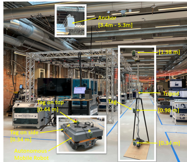
Figure 1. Picture of the AAU 5G Smart Production Lab showing: a tripod with three tag heights (static use case), an AMR with tags on its sides and top surface (mobile use case), and one of the anchors.
