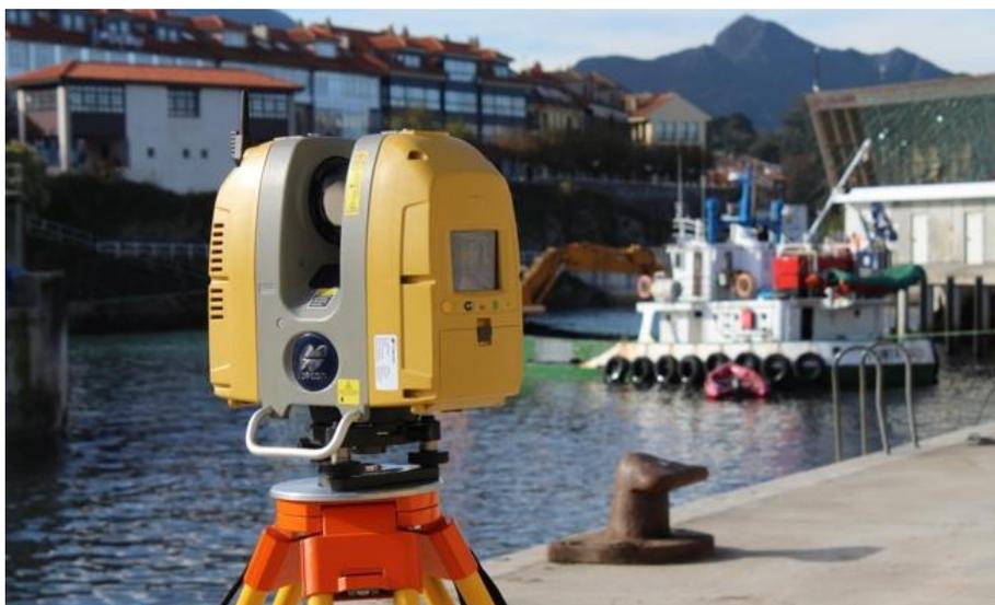
Figura 15. LiDAR terrestre GLS 2000 [Excade SL]
