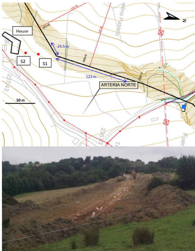
Fig. 4. Location of the seismographs and pipeline trace (upper) and trench viewed from S1 (lower).
