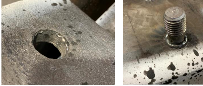
Figure 16. Burring effect in the hole of the cleat
