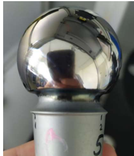
Figure 74. Location and position of the ball stud in the Opto-Shaft TT machine
