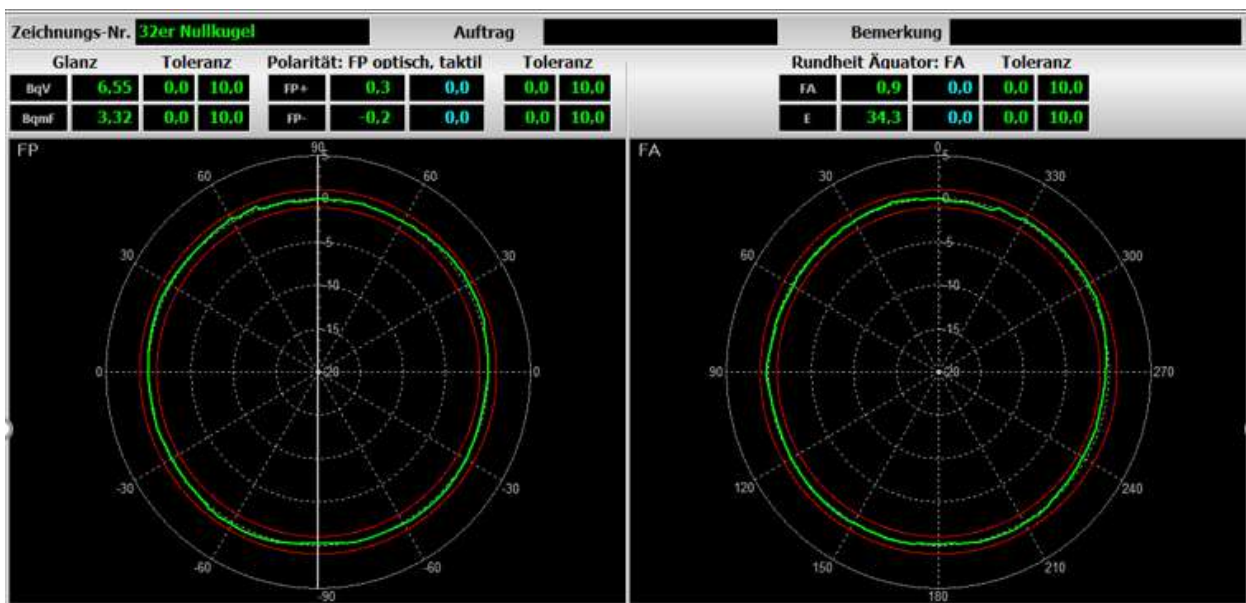
Figure 949. Comparison between optic and equator measures
