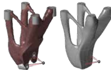
Figure 2. Optimization (a), Post-processed geometry (b).
