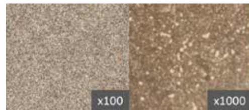
Figure 2. Martensitic microstructure of one of the samples (x100 and x1000)
