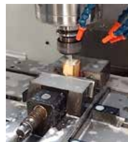
Figure 1. Embedded Macor ® block during machining.
