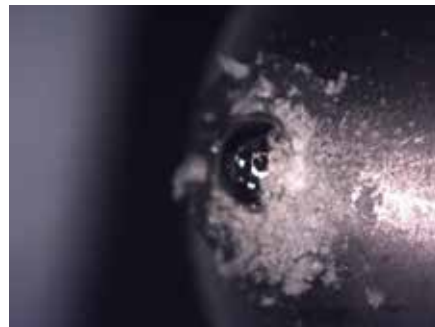
Figure 1. Wear debris of friction tests on Pin
