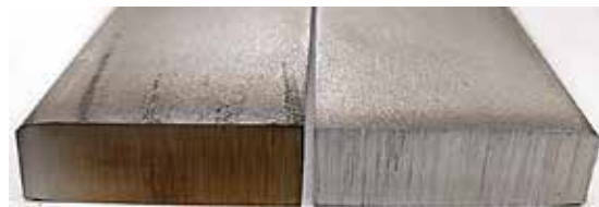
Figure 2. Thermal damage on test pieces using different process conditions.
