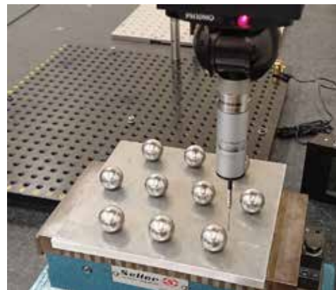
Figure 1. Contact measurement of a set of ten spheres (25 mm diameter).
