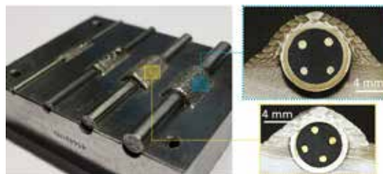
Figure 1. MI cables embedded by LMD
