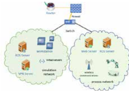
Figure 1. Communications architecture for industrial environments under cybersecurity requirements
