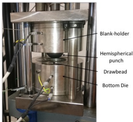
Figure 1. Experimental Nakazima test device developed.
