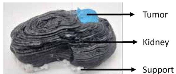
Figure 1. 3D printing of a prototype using a hybrid multi-material 3D printing which can use both hard and soft materials as well as different colours at the same time.
