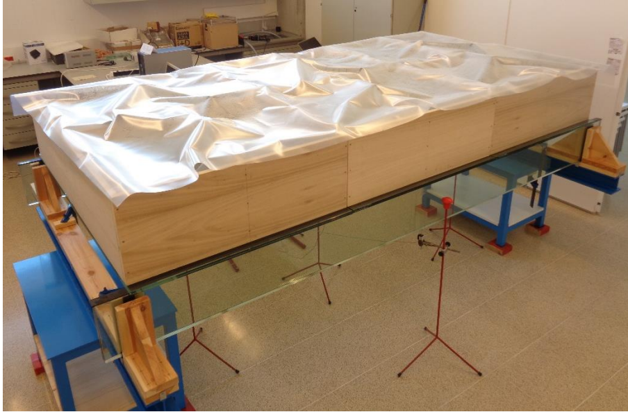
Figure 12. Laminated glass slab loaded with water and covered with a polymeric film to prevent water evaporation.
