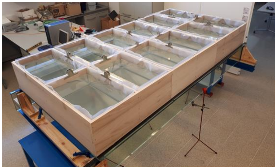
Figure 11. Laminated glass slab with the full load of water poured into the 12 compartments of the wooden formwork, with plastic bags to prevent water leakage.
