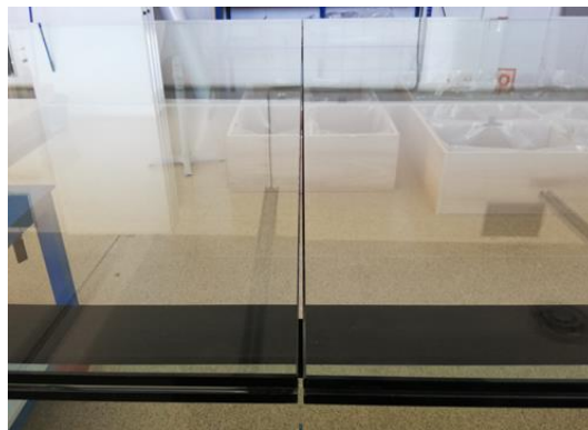
Figure 5. Separation between laminated glass plates.
