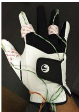
FIGURE 1. Glove used for vibrotactile stimulation.
